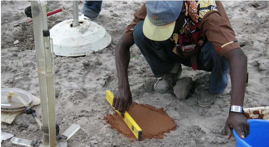
Figure 2.2 To enable hydraulic contact underneath the entire disc, moist sand was applied and made horizontal with a water pass.
