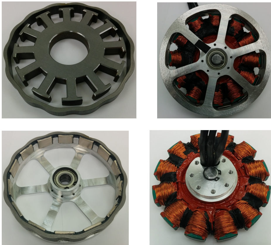
Figure 3.32: Final EV motor prototype that uses the 14 pole - 12 slot configuration to improve the motor core losses.
