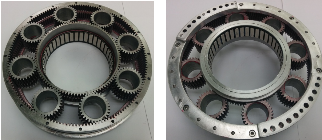
Figure 6.4: High reduction (1 : 101) bearingless planetary gearbox. Similar to Fig. 6.1 the rotor of the driving outrunner is built-in the driving sun gear.
