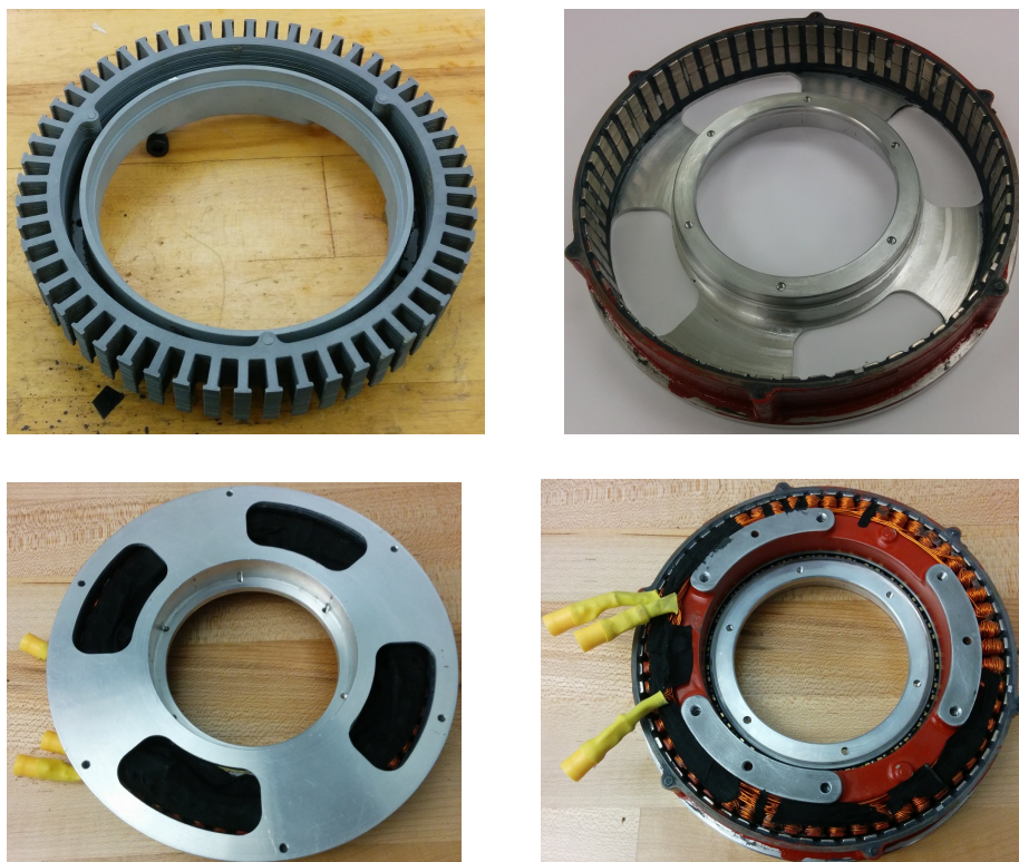
Figure 3.34: Robotics motor prototype that has 60 poles and 54 slots.
