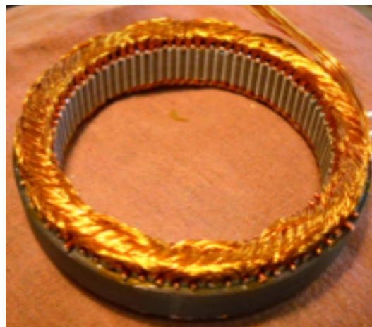
Figure 3.5: Stator of distributed winding frameless motor [30] ©2015 IEEE.
