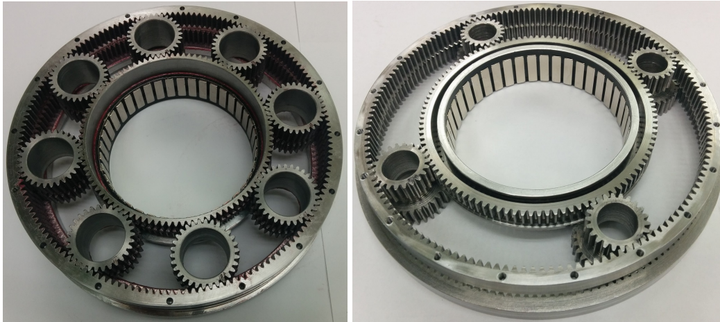
Figure 4.22: Prototype of the bearingless planetary gearbox with no planet assembly features. The gearbox on the left is a remake of the gearbox of Fig. 4.12 with substantially lower backlash and is used in the actuator prototype of Sec. 6.3. The gearbox on the right has reduction ration of 1 : 10 and is used in the actuator prototype of Sec. 6.2.
