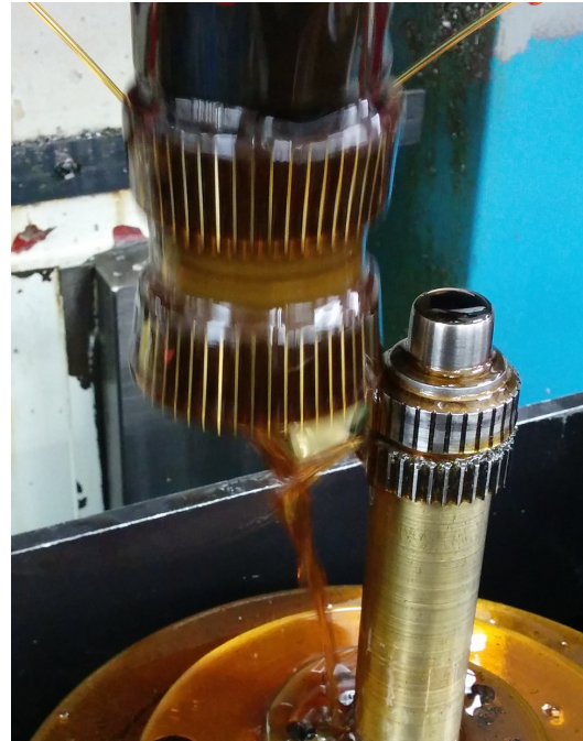
Figure 4.21: Compound planet manufacturing using double-sided shaping.
