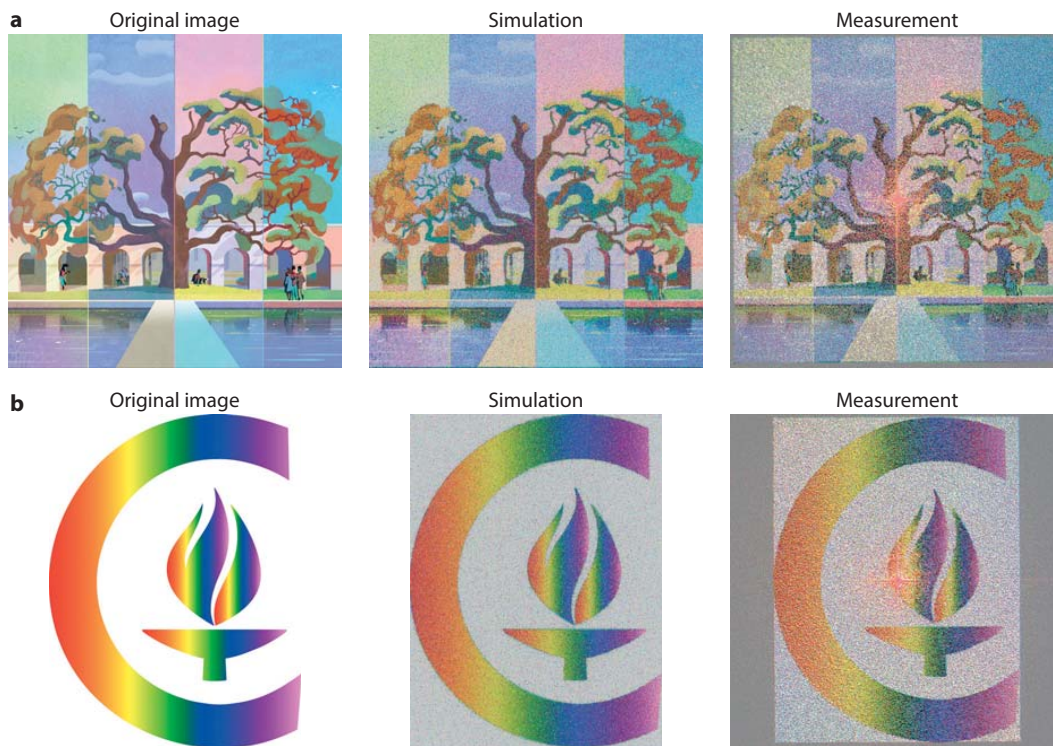
Figure 2.9: Simulation and measurement results (a) and (b) The original target image along with simulated and measured polarization holograms converted to false-color images. Both holograms are about 30-degrees tall, corresponding to a diagonal NA of 0.36 for the holograms in panel a.
