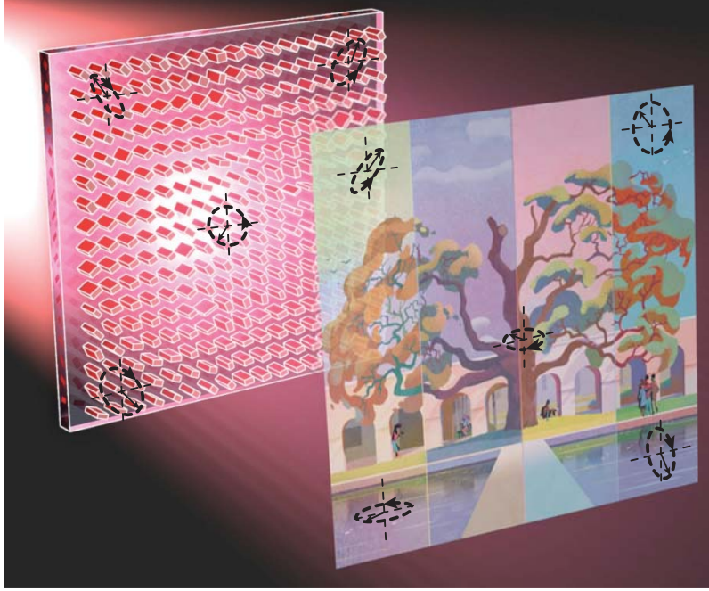
Figure 2.5: Schematic illustration of a metasurface polarization hologram, projecting a polarization pattern encoding an RGB image. The metasurface is illuminated with a beam of known wavelength and polarization. Each dielectric nano-post is designed to control the polarization and phase of the output light at the corresponding lattice site.
