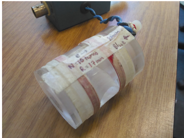
Figure D.5: Image of Helmholtz coil ( N=10 , R=17 mm) used for calibration of probe array. The coil is wound on a machined plastic cylinder with a 14 mm axial hole and a 14 mm perpendicular hole for calibrating the other two axes.
