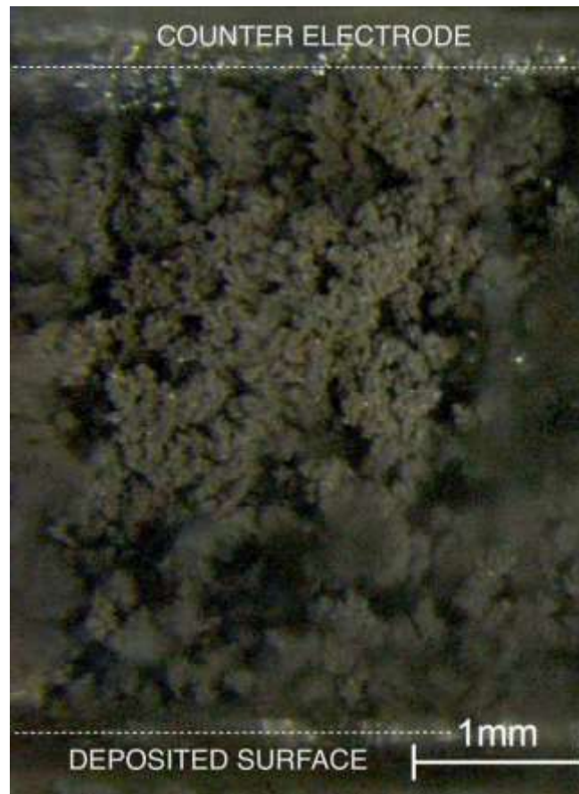
Figure 1' : Observed dendrites which reach the counter electrode and short the cell.
