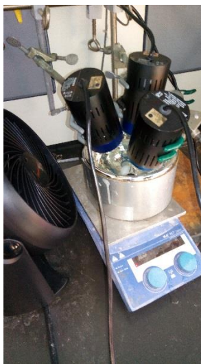
Figure 3.19. A typical irradiation setup at room temperature. Shown are three 34-watt blue LED lamps, a reflective Dewar, and a table fan.
