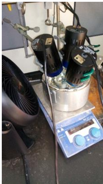
Figure 4.4. A typical irradiation setup at room temperature. Shown are three 34-watt blue LED lamps, a reflective Dewar, and a table fan.
