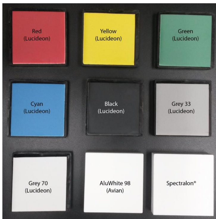
Figure 4. Calibration targets used in this study with manufacturer indicated in parentheses and Spectralon® for comparison. All of the Lucideon targets are mounted on a black plastic holder. The AluWhite 98 target is not mounted on any material.
