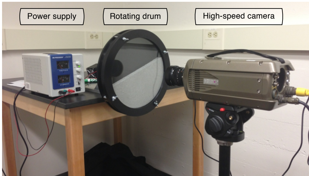
Figure 2.2: Experimental setup for studying granular flow in a rotating drum
