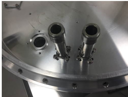
Figure A.6: Corrected clocking of the fore bulkhead cryostat fill tube mounting holes. Here, the cryostat fill tubes were successfully installed.
