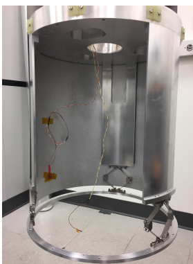
(b) Flexures in an intermediate stage of CIBER-2 assembly. The skin ring is visible at the bottom of the image.
