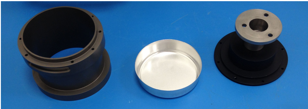
Figure A.18: Detector support pieces; from left, Titanium can, Molybdenum support mounted to anodized Aluminum base (black). In center, a cup for screws used during assembly.
