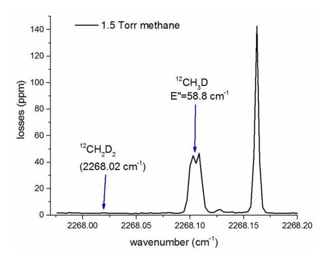
**Figure S4. 2.** Broadband measurement of a 1.5 Torr methane sample between 2267.925 cm<sup>-1</sup> and 2268.20 cm<sup>-1</sup> showing the line position and relative strength difference of the lines used for  $^{12}\text{CH}_2\text{D}_2/^{12}\text{CH}_3\text{D}$  measurement.
