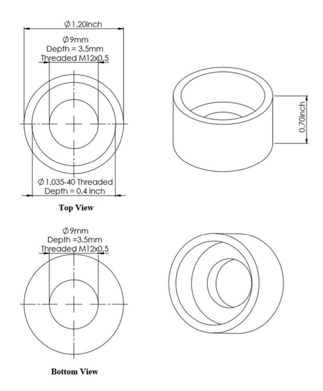
Figure S2.17. 1 inch mirror mount detail.
