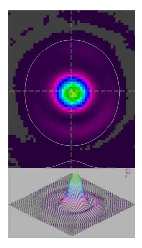
**Figure S2.3.** Beam profile of the collimated laser beam measured 57 inches away from the laser, with only an anti-reflective (AR) coated aspheric lens (Lightpath 390036-IR4) with a focal length of 3.05 mm. The beam diameters in the X and Y dimensions are 2.16 mm and 2.22 mm, respectively
