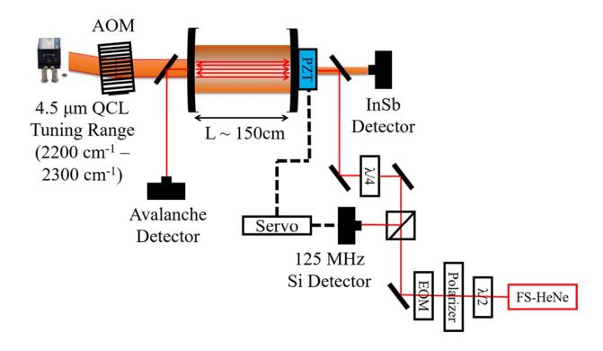
**Figure 4. 1.** Schematic of the FS-CRDS instrument for doubly substituted methane isotope composition measurements.
