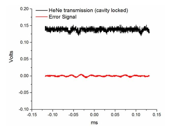
**Figure S4. 1.** Performance of the PDH locked cavity. The black trace is shows the HeNe transmission signal detected on the avalanche detector. The red trace shows the error signal produced from the lock-in amplifier
