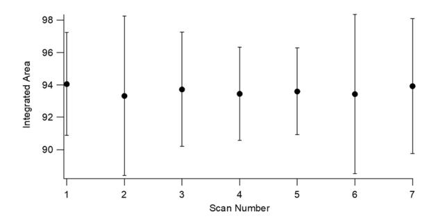
**Figure S4. 3.** Fitted area of the 7 <sup>12</sup>CH<sub>3</sub>D lines. Error bars shown in this figure came from the reported error in the fit results.
