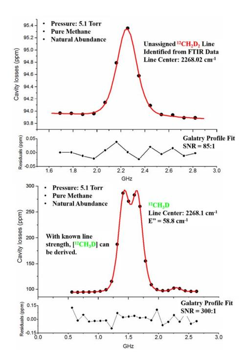
**Figure 4. 6.** Sample spectra of a pair of the <sup>12</sup>CH<sub>2</sub>D<sub>2</sub> and <sup>12</sup>CH<sub>3</sub>D abundance measurement of a 5.1 Torr natural abundance methane measurement. The black dots in each spectrum was the measured data and the red solid line is the fitted model. Both spectra were fitted to Galatry profiles with residuals shown in the figures.
