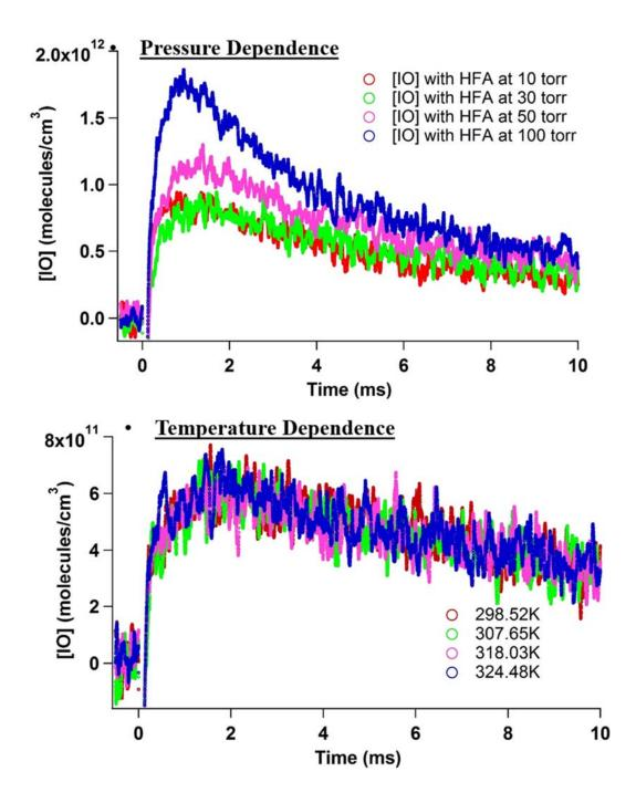
**Figure. 5. 7.** Pressure and temperature dependence of the IO profile was also measured. There was no temperature dependence for the IO kinetics. There is a positive dependence for the IO production, indicating a negative pressure dependence for CH<sub>2</sub>OO production, since the overall CH<sub>2</sub>I + O<sub>2</sub> reaction is pressure independent.
