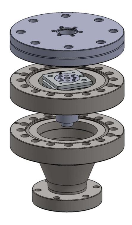
Figure S2.12. Laser side ring-down mirror mount detail.
