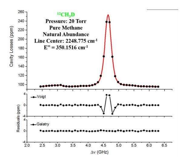
**Figure. 4. 4.** Comparison of the Viogt profile versus Galatry profile model for the <sup>12</sup>CH<sub>3</sub>D spectrum at 2248.75 cm<sup>-1</sup> from measurement of a 20 Torr natural abundance methane sample. In the upper panel, the measured data are shown in the black dots, while the red solid line is the galatry profile fit. The middle and bottom panels are the residuals for these two profile fits.
