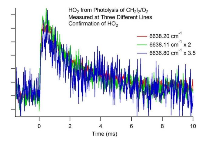
**Figure. 5. 3.** HO<sub>2</sub> was observed from the CH<sub>2</sub>I<sub>2</sub>/O<sub>2</sub> system. The product was confirmed to be HO<sub>2</sub> by measurement at different HO<sub>2</sub> transitions.
