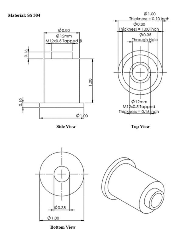
**Figure S2.16.** Flexure mount to mirror mount extension mount. This was designed to replace a Piezo which was originally used for an FS-CRDS design.
