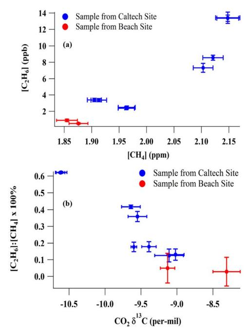
**Figure 2.5.** Results from measurements of 10 ambient air samples, including 8 of the Caltech site samples and 2 of the beach site (PV site) samples. (a) Ethane abundance as a function of methane. (b) Ethane to methane ratio as a function of the isotope content of the carbon dioxide in the same sample.
