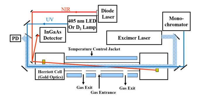
**Figure. 5. 2.** Schematic of the infrared kinetics spectroscopy (IRKS) apparatus showing the three light sources.
