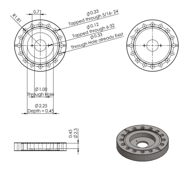
Figure S2.14. Modified 4.5 inch double sided flange for flexure mount mounting.
