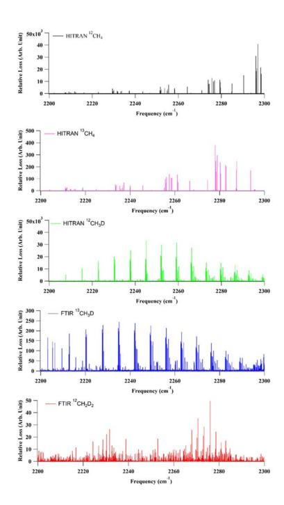
**Figure. 4. 3.** Absorption line positions and relative strength for five of the major isotopologues of methane within the tuning range of the EC-QCL laser used for our spectrometer. Spectra of the first 3 isotopologues were generated based on the line parameters reported in the HITRAN database. Spectra of the two doubly substituted methane isotopologues were from normalized high resolution FTIR measurements of pure <sup>13</sup>CH<sub>3</sub>D and <sup>12</sup>CH<sub>2</sub>D<sub>2</sub>.
