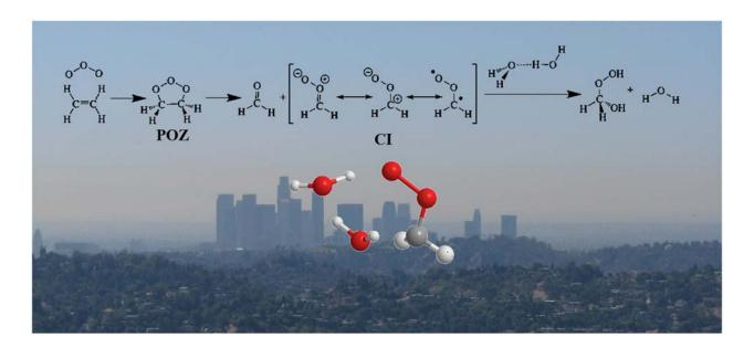
**Figure. 5. 1.** Schematic of the reaction mechanism of the oznolysis reaction mechanism of the smallest alkene.
