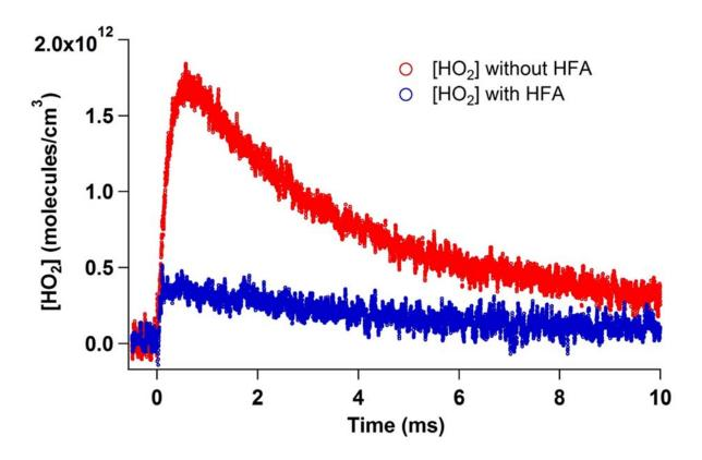
**Figure. 5. 4.** Hexafluoroacetone (HFA) was added as a Criegee scavenger to study reaction kinetics with or without CI. It was found that most of the HO<sub>2</sub> was made from CI, while there is a fast HO<sub>2</sub> formation mechanism unrelated to CI, most likely from direct CH<sub>2</sub>I + O<sub>2</sub> reaction.
