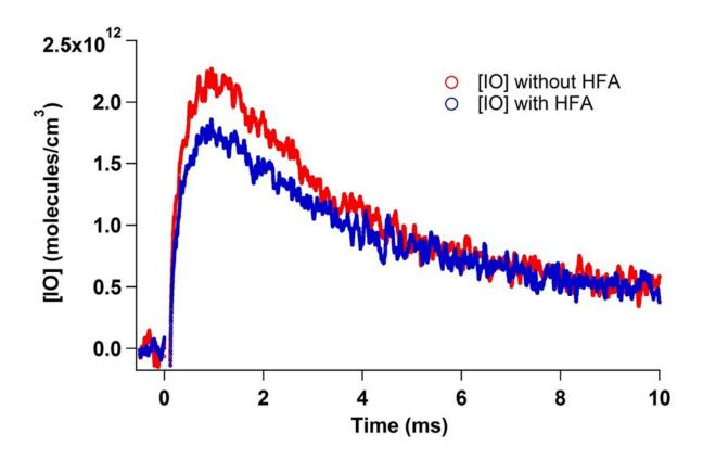
Figure. 5. 5. We also monitored IO simultaneously with HO<sub>2</sub>. IO was made mainly from  $CH_2IOO + I$ . The rate for this reaction was about  $4 \times 10^{-11}$  cm<sup>3</sup>molecules<sup>-1</sup>s<sup>-1</sup>. From the experiments with HFA, we found that some of the IO came from the reaction between  $CH_2OO$  and I.
