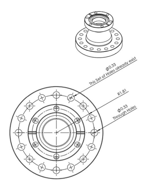
Figure S2.13. Modified 2.75 inch CF to 4.5 inch CF conical reducer detail.
