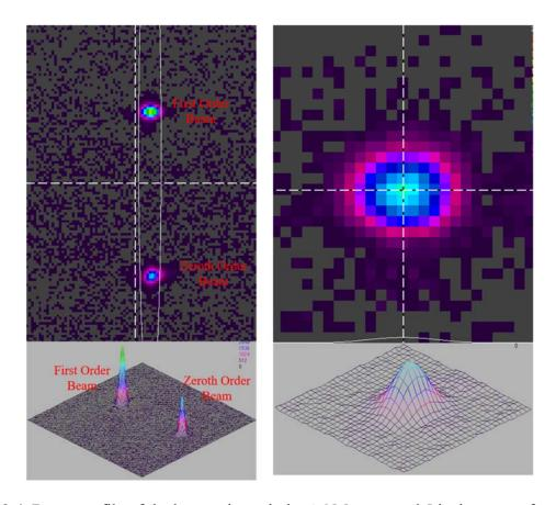
**Figure S2.4.** Beam profile of the beams through the AOM measured 5 inches away from the AOM output. The left panels include both the zeroth order (transmitted) and the first order diffracted beam, with the more intense beam as the first order beam. The right panels are the zoomed in observation of the first order beam. The beam diameters in the X and Y dimensions are 0.37 mm and 0.25 mm, respectively.
