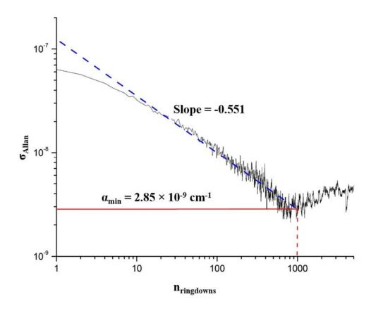
**Figure 2.2.** Allan deviation plot for the ringdown decays of vacuum baseline losses at 2976.788 cm<sup>-1</sup>. The acquisition rate is  $\sim 20$  Hz with the estimated minimum detectable absorbance of the spectrometer as  $2.85 \times 10^{-9}$  cm<sup>-1</sup>.
