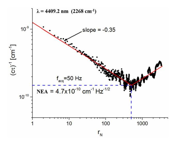
**Figure 4.2.** Allan deviation plot for the ringdown decays of vacuum baseline losses at 2268.00 cm<sup>-1</sup>. The acquisition rate is  $\sim 50$  Hz with the estimated minimum detectable absorbance of the spectrometer as  $1.49 \times 10^{-10}$  cm<sup>-1</sup>.
