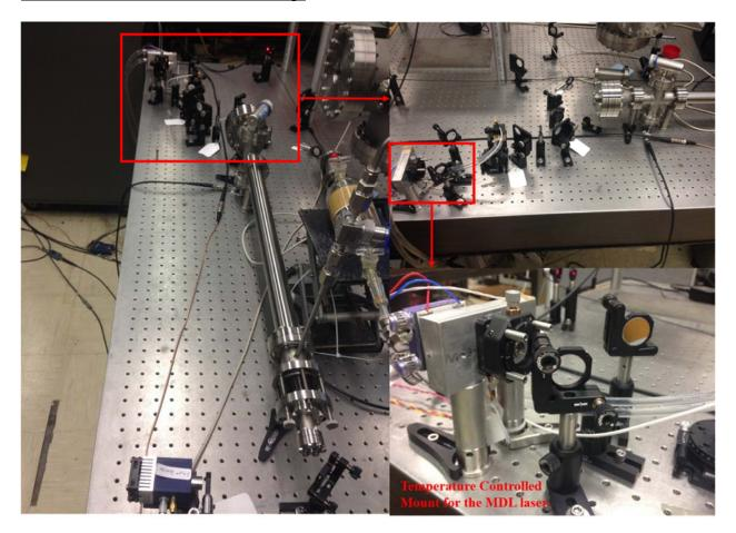
**Figure S2.11.** Picture of the CRDS cavity spectrometer and the zoomed in view of the temperature controlled ICL mount.
