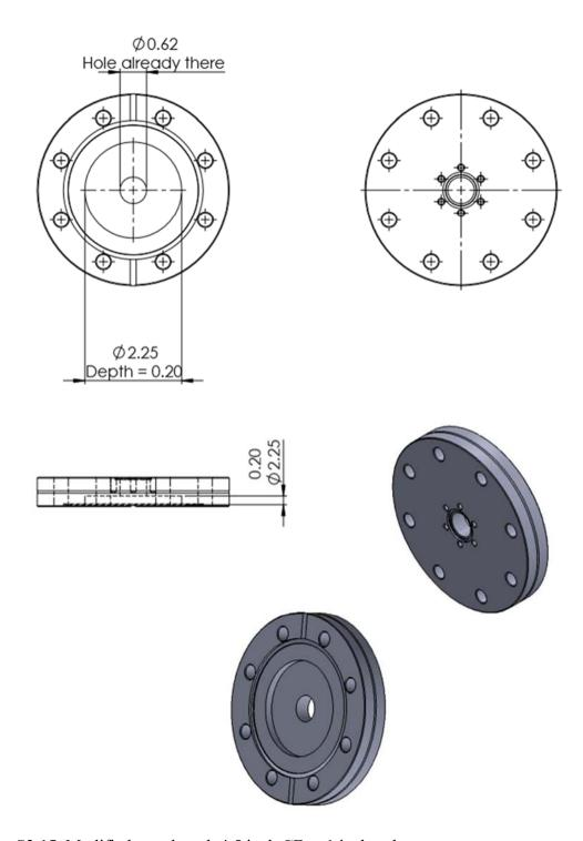
Figure S2.15. Modified zero length 4.5 inch CF to 1 inch reducer.
