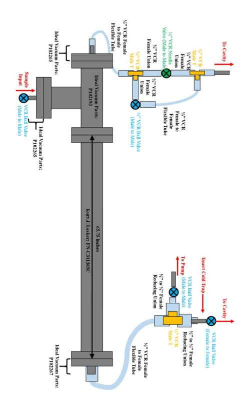
Figure S4. 6. Schematic of the sample inlet design configuration.
