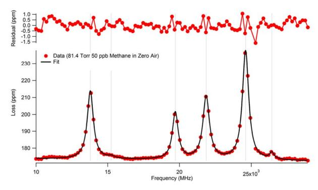
**Figure S2.5.** Measurement of 50 ppb methane between 2978.4 cm<sup>-1</sup> and 2979.2 cm<sup>-1</sup>. Total pressure of the cavity was 81.4 Torr. The cavity FSR was varied to fit the data (red dots) to the HITRAN simulated spectrum (black trace). The top panel is the residual between the data and the fit. The calculated FSR is 182.5 MHz, resulting in a calculated cavity length of 82.2 cm.
