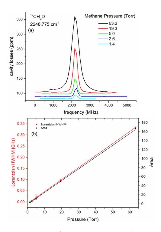
**Figure. 4. 5.** Lineshape study of the <sup>12</sup>CH<sub>3</sub>D line centered at 2248.775 cm<sup>-1</sup>. (a) Spectra of the <sup>12</sup>CH<sub>3</sub>D transition measured at pressures between 1.4 Torr and 63.2 Torr. (b) Spectral fit results, Lorentzian width (HWHM) and integrated area, plotted as a function of the total methane pressure.
