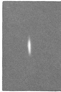
(a) Point Focus (Enlarged 5.8 times) 3 minute exposure at 20 PKV and 20 MA with beam in air.
