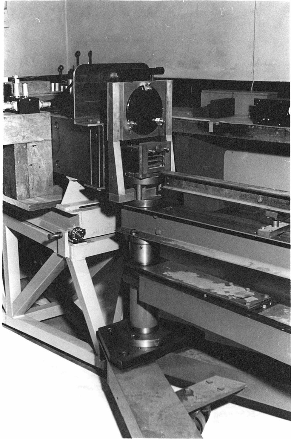
Fig. 18 - Showing the permanent provision now made for mounting the 6" concave mirror above the crystal holder. Using the mirror and its corresponding microscope, the minute deflections due to the bending of the  $1\frac{1}{4}$  inch bar can be measured whenever line profiles are being delineated.
