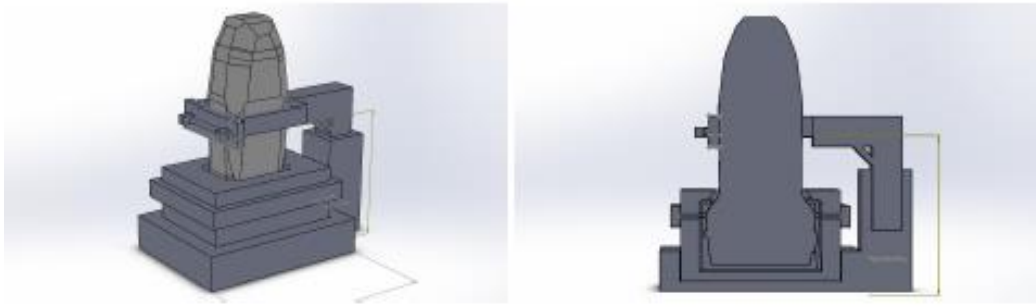
Figure 3. 3 Mold for manufacturing the ultrasound pressure sensor [40]
