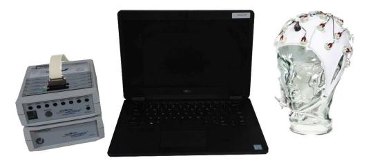
Figure 3.1 - ActiChamp Amplifier with ActiCap active electrodes
