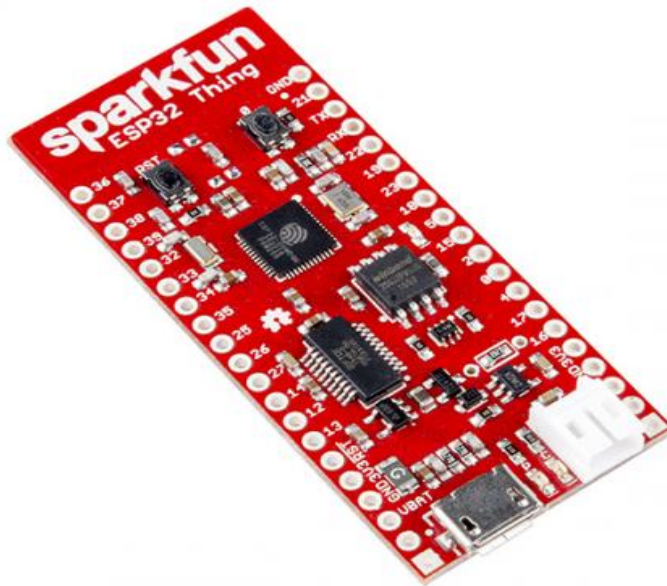
Figure 3- 2: SparkFun ESP32 Thing [34]
