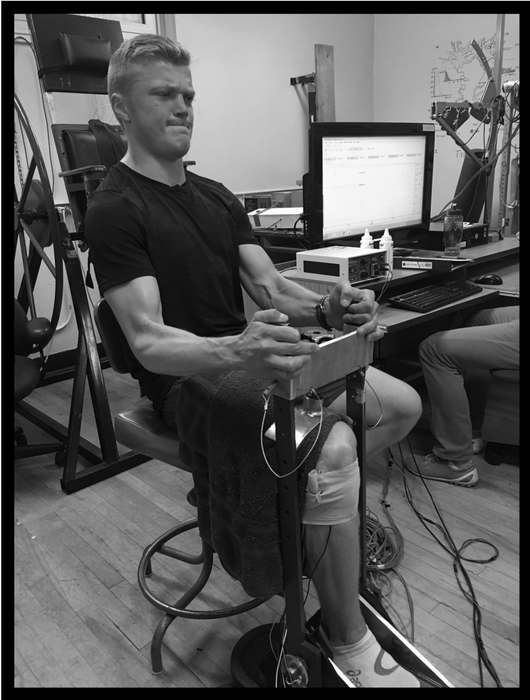
Figure 3.12. Experimental set-up and method for measuring plantar flexors MVC using the boot apparatus.
