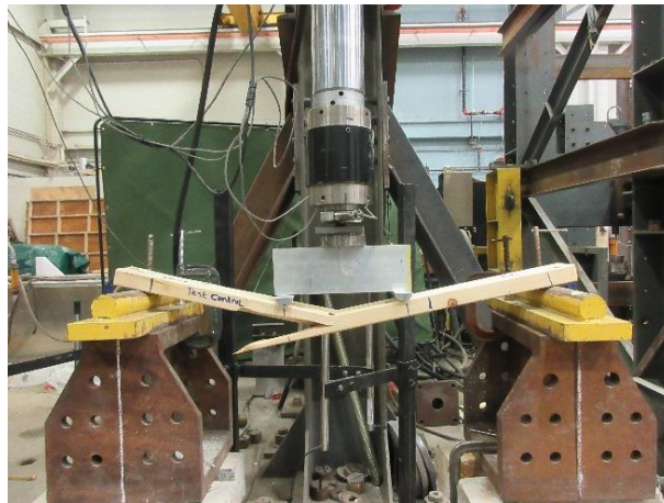
Figure 5 Failure of the experimental control spruce specimen (without FJ)
