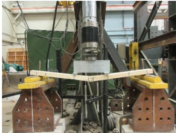
Figure 11 Experimental test of spruce specimen with FJ
