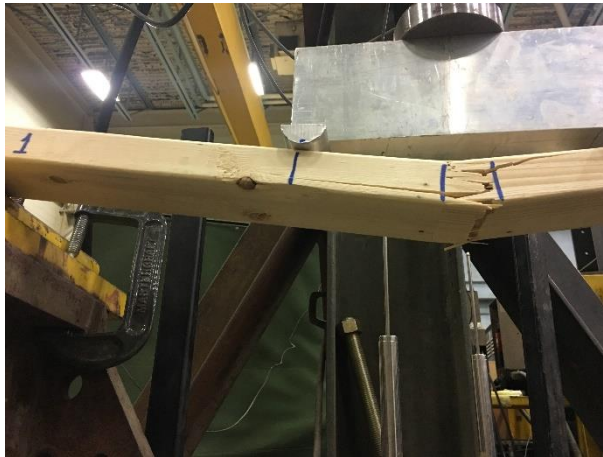
Figure 12 Failure of the experimental spruce specimen with FJ
