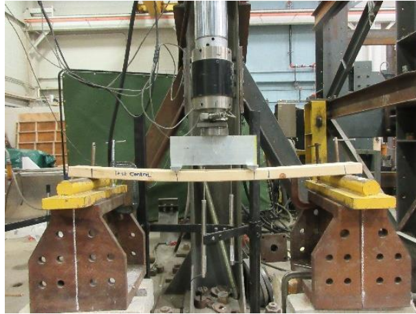
Figure 4 Experimental test of control spruce specimen (without FJ)
