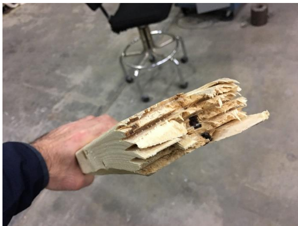
Figure 13 Failure profile of the spruce specimen with FJ
