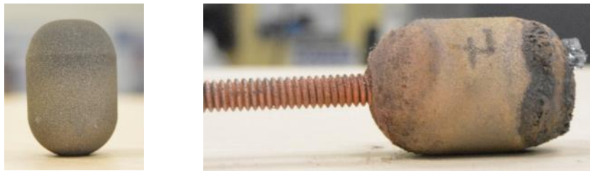
Figure 16: Sample #3 before and after immersion tests
