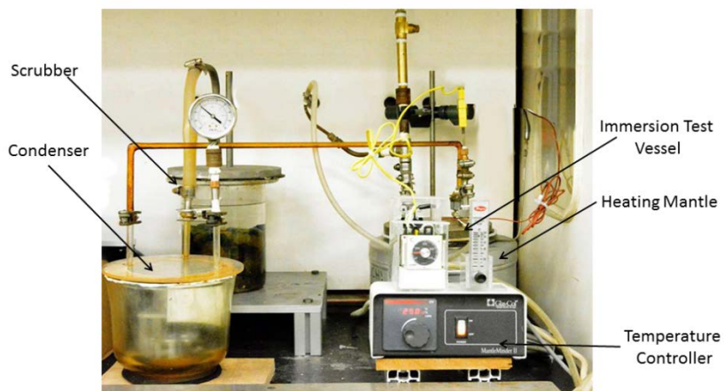
Figure 13: Experimental apparatus for coatings evaluation
