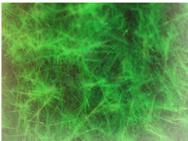
Figure 6: Configuration of crystalline solid (green dendrites) at temperatures below room temperature
