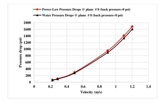
Figure 4.21: Velocity and pressure drop relationship at back pressure 0 psi at plane #8
