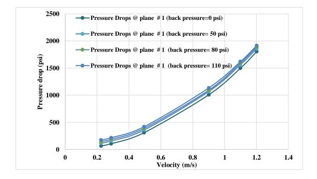
Figure A. 23: Relationships between fluid velocities and pressure drops at plane #1
