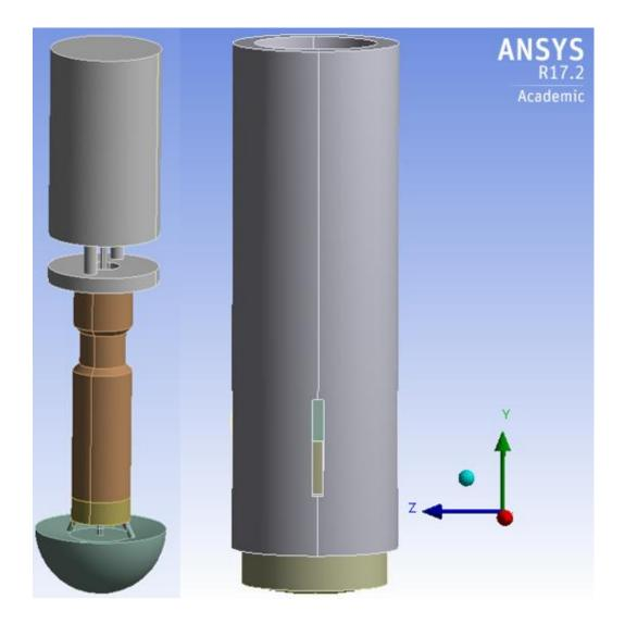
Figure 4.3: Thruster geometry simulated by ANSYS
