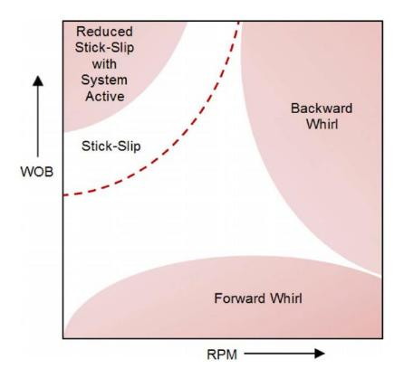
Figure 2.2: Drilling path and vibration types (Dunlop et al., 2011)
