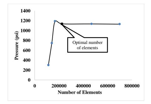
Figure 3.6: Number of elements and the represented pressure for best Thruster meshing
