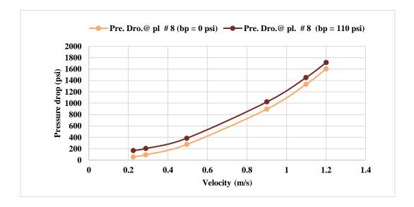
Figure 4.18: Relationships between fluid velocities and pressure drops at plane # 8, which is located at the chocking region of the Thruster at 2 different back pressures including 0 psi
