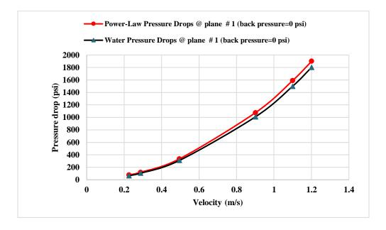
Figure 4. 20: Velocity and pressure drop relationship at back pressure 0 psi at plane #1
