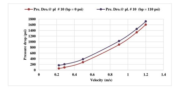
Figure 4. 19: Relationships between fluid velocities and pressure drops at plane #10, which is located prior to fluid exit from the Thruster at 2 different back pressures including 0 psi
