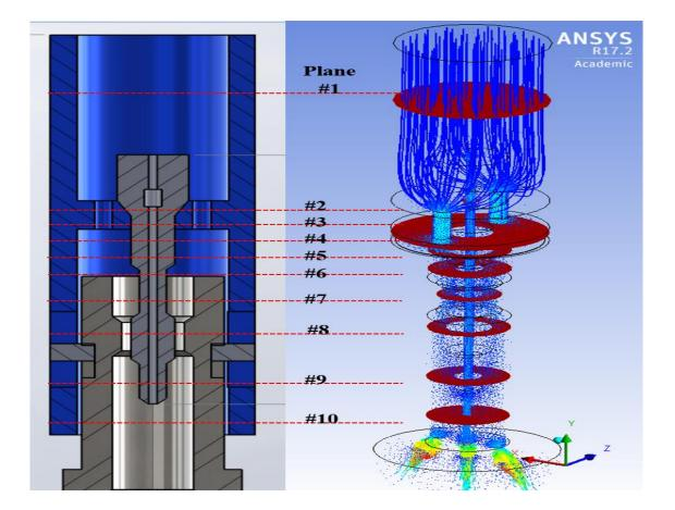
Figure 4. 15: Planes at various locations throughout the Thruster for velocity and pressure drop analysis
