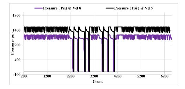
Figure 4.14: The relationship between various inlet fluid velocities and the resultant pressure effect
