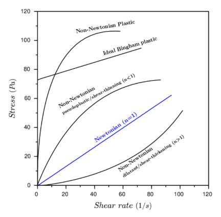
Figure 2.1: Classifications of fluids from Newtonian and non-Newtonian (Irgens, F., & SpringerLink, 2014
