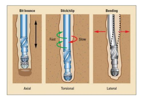
Figure 2.3: Drillstring vibration models (Zamani, 2016)
