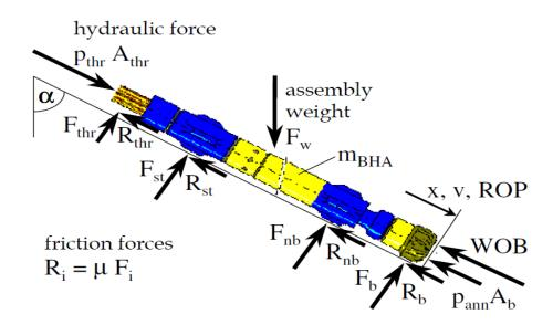
Figure 3.1: Free body diagram of a floating thruster as a part of the BHA
