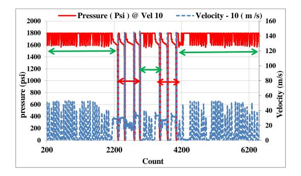
Figure A.18: Combined pressure and velocity profiles for full length of Thruster. Green: Pre and Post chocked regions, Red: Unchoked region
