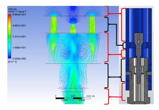
Figure 3.7: ANSYS fluent R 17.2 fluid flow simulation of the Thruster
