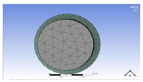
**Figure 3.5: Meshing of the Thruster**
