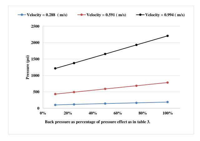
Figure 4.9: Thruster generated pressure as percentage back pressure of the pressure affect
