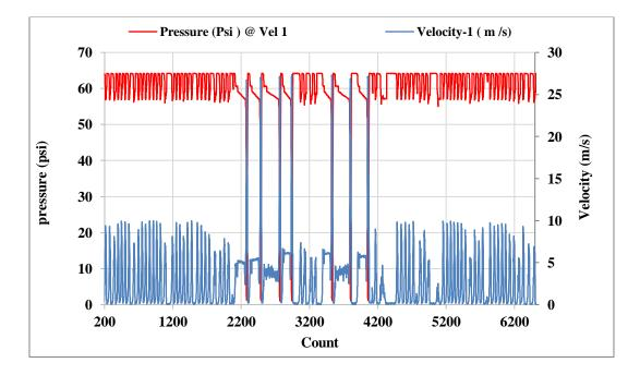
Figure 4.12: Combined pressure pulse at the input velocity 1 as a result of the Thruster operation under this condition
