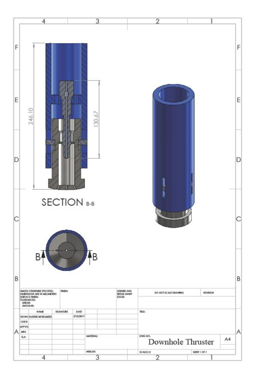
Figure A.1: AutoCAD drawing of the Thruster
