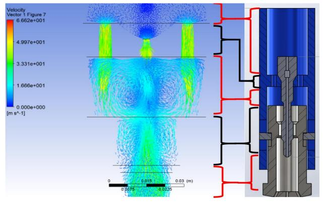
Figure 4.6: ANSYS Fluent 17.2 fluid flow simulation of the Thruster
