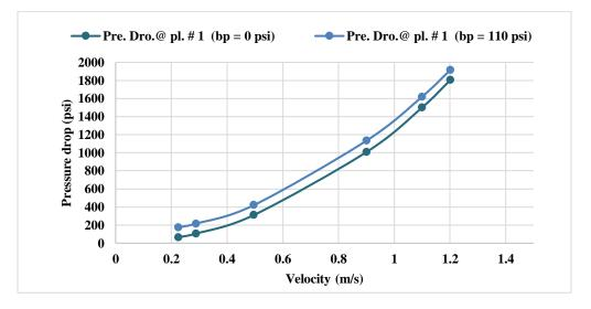
Figure 4. 17: Relationships between fluid (water) velocities and pressure drops at plane #1, which is located at the entrance of the Thruster at 2 different back pressures including 0
