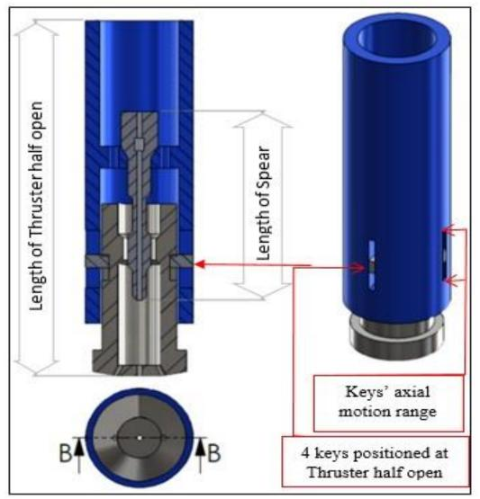
**Figure 4.1: Drawing of the Thruster**
