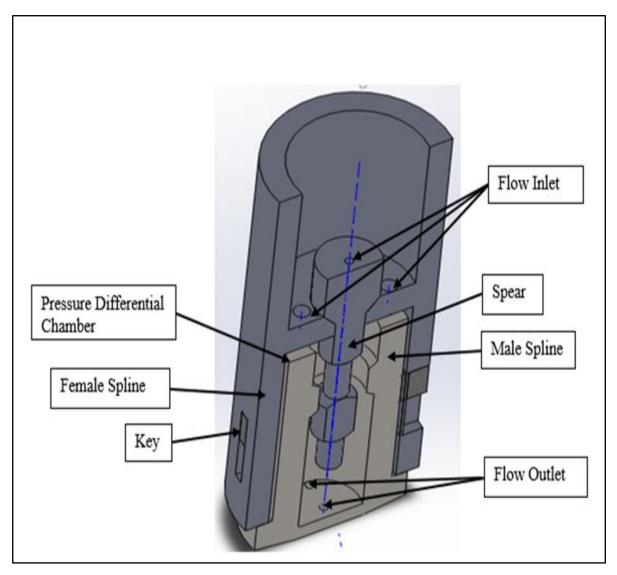
Figure 4.2: Thruster mechanical design
