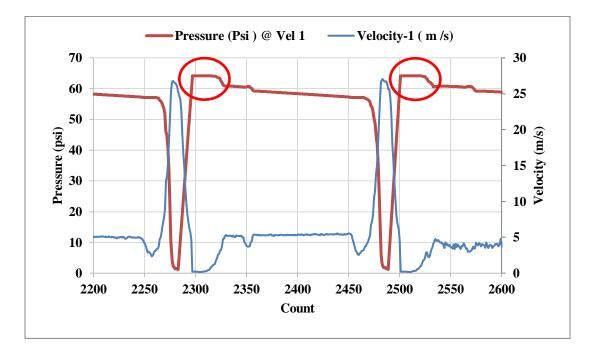
Figure A.19: Pressure and velocity fluctuation inducing axial motion of the Thruster. After the drop, the pressure gains some increase compared to the pre-drop stage pressure
