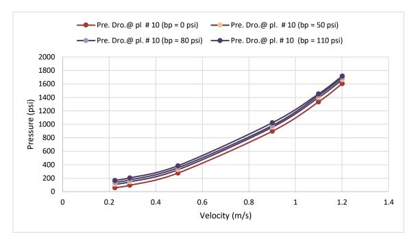
Figure A.25: Relationships between fluid velocities and pressure drops at plane #10
