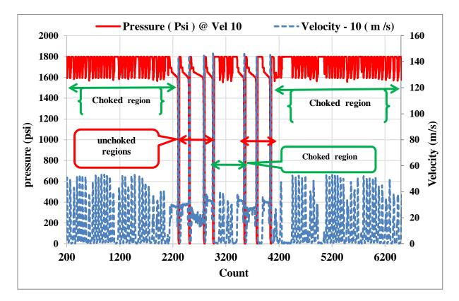
Figure 4.13: Thruster pressure pulse at velocity 10 with Choked and unchoked regions
