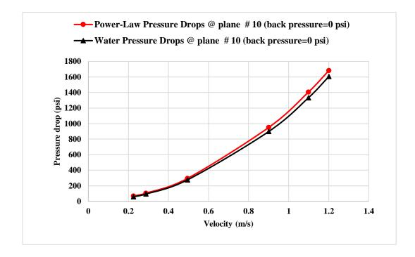
Figure 4. 22: Velocity and pressure drop relationship at back pressure 0 psi at plane #10
