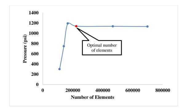
Figure 4.5: Number of elements and the representative pressure for best Thruster meshing
