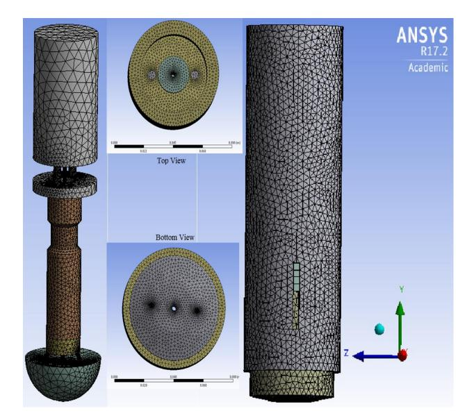
Figure 4.4: Thruster meshing
