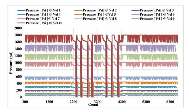
Figure A.20: Relationship between 10 pressure profiles and 10 corresponding flow rates
