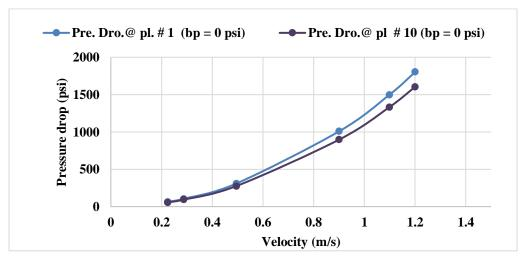
Figure 4.16: Relationships between fluid (water) velocities and pressure drops at plane #
