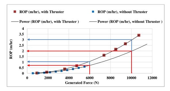
Figure 4.8: The resultant ROP in both applications based on Maurer Model for with and with no Thruster
