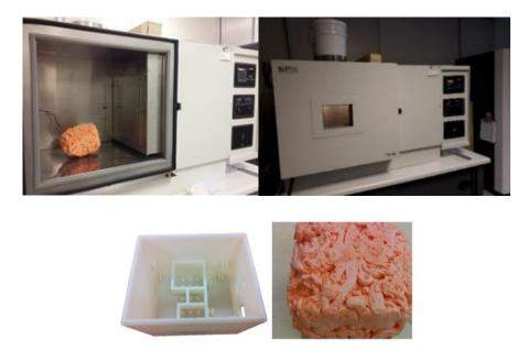
Figure 5-16 Cold chamber setup and the enclosure prototype with an insulation layer.
