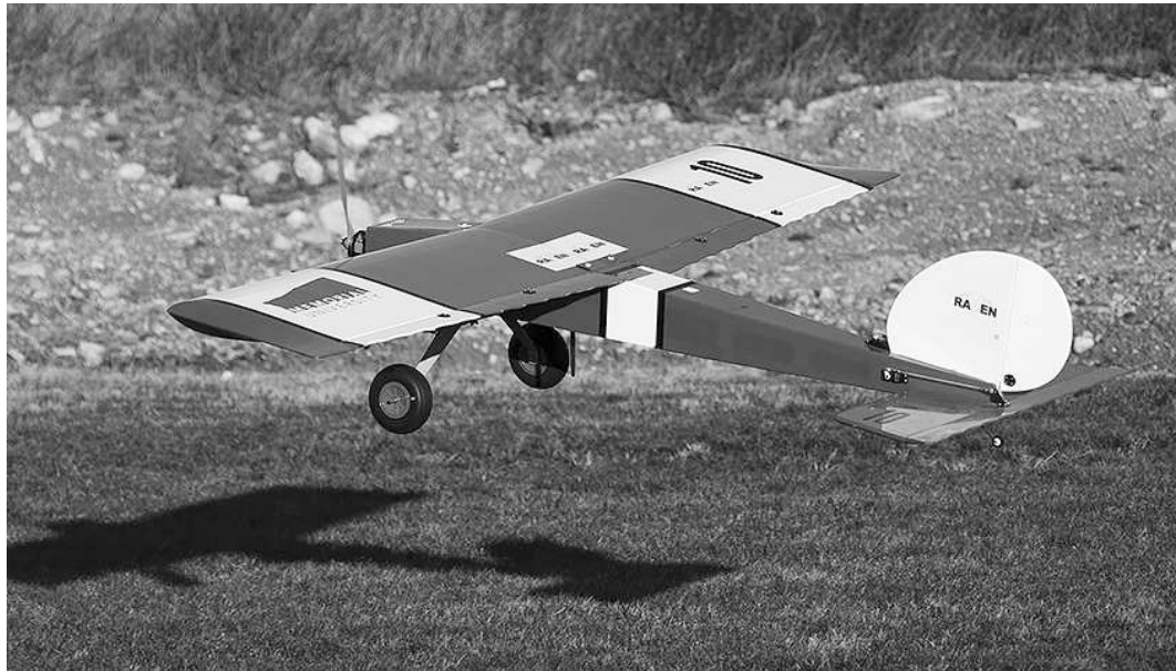
Figure 5.2: Giant Big Stik model aircraft configured as UAV.
