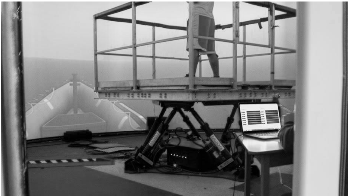
Figure 3.1: Data collection set-up showing the 6 DoF motion platform and the screen of the simulator. The bow of the simulated FRC is visible on the screen.
