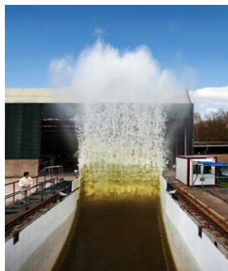
Fig. 1-2 The behavior of spray formation and spray cloud at different heights was not a concern. The impact pressure was studied. (Sloshel Project, Brosset et al. , 2009).
