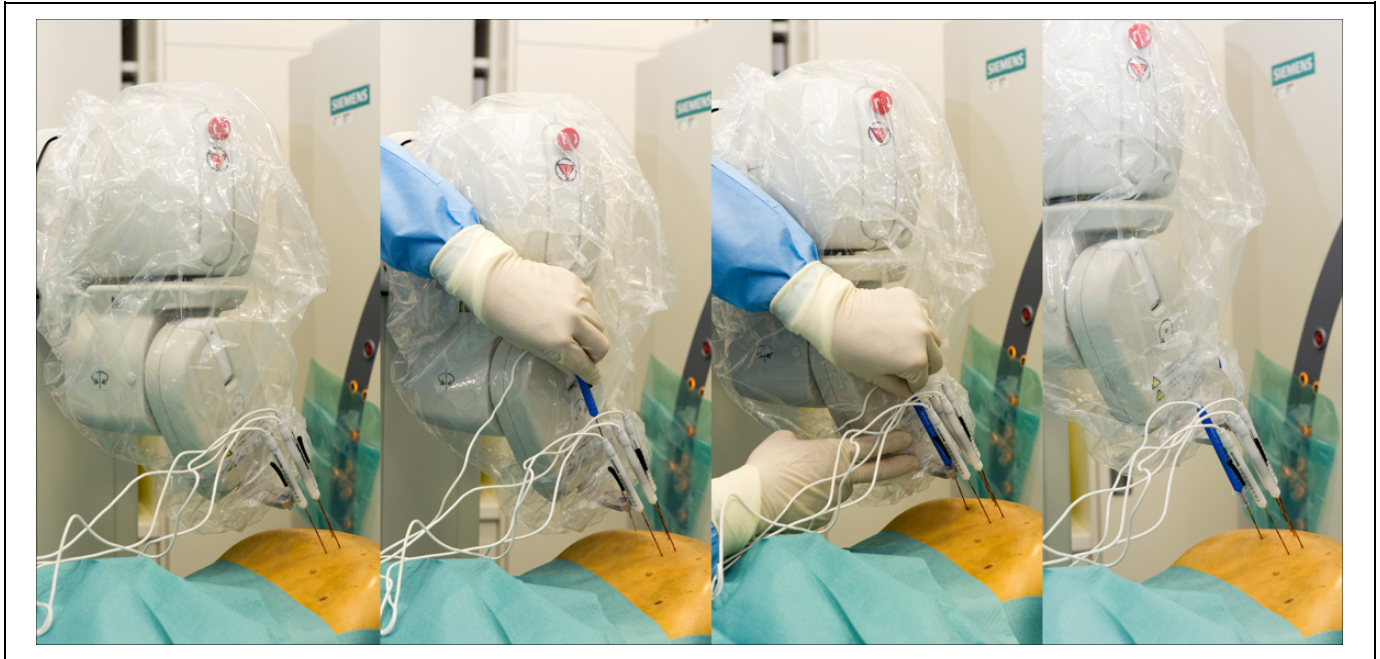
Figure 3. Robot-assisted irreversible electroporation (IRE) of a liver metastasis. The robotic arm positions itself according to the predefined plan (A) and the physician applies the probe through the probe guide (B and C). The robotic arm moves to the position of the next electrode (D; using MAXIO Perfint Healthcare).
