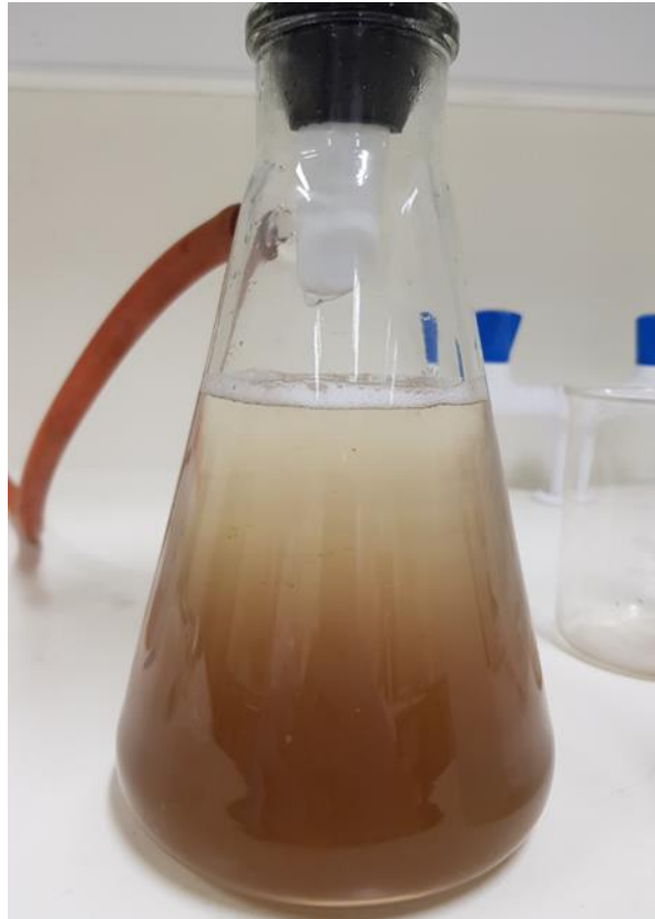
Figure 41: Washate from test 3, displaying a clear separation occurring within the flask
