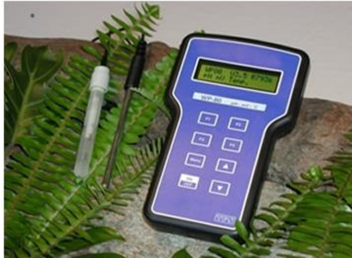
Figure 49: TPS's WP-80 pH- MV- Temperature meter ENREF 75 TPS Australia (2018).
