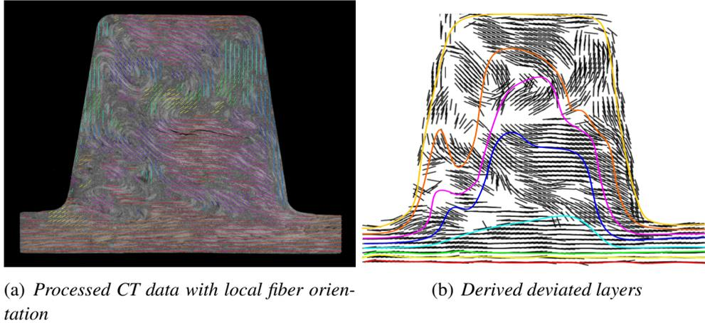
Figure 3 – Out of plane fiber orientation for a rib cross section with an aspect ratio of 0.67 (width to height).
