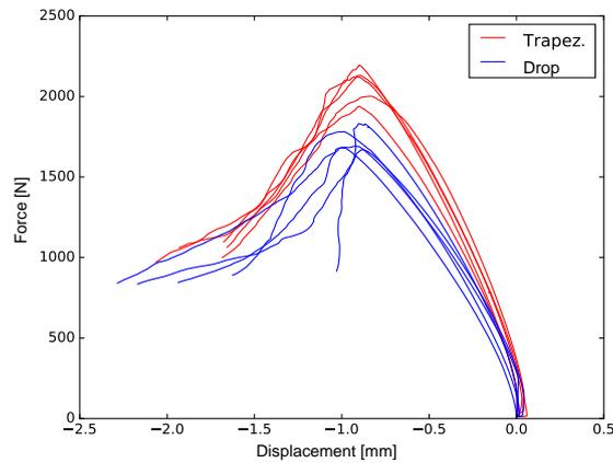
Figure 6 – Four point bending test results of rib specimen with 0.67 aspect ratio.
