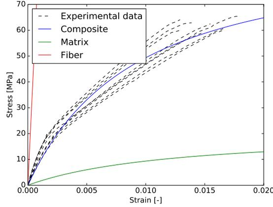
Figure 1 – Inverse determination of the nonlinear matrix properties.
