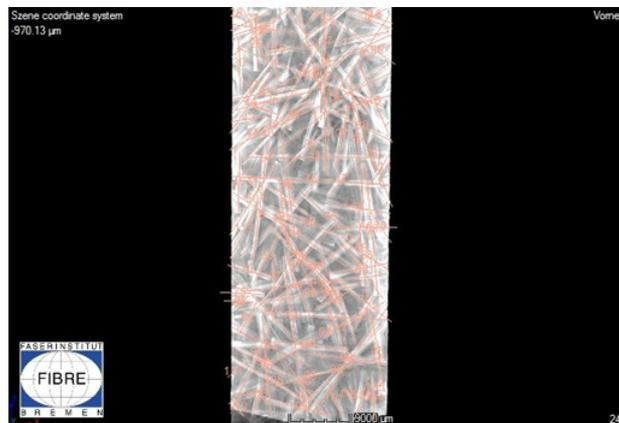
Figure 2 – In plane fiber bundle orientation.
