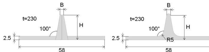
Figure 5 – Definition of trapezoidal and drop rib specimen (measurements in mm).
