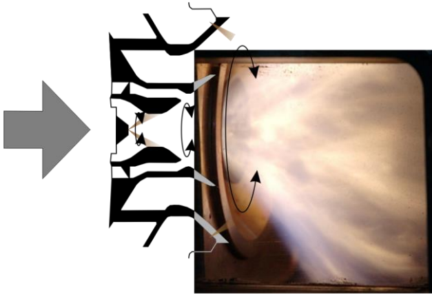
Fig. 1: Schematic of the fuel injector, including pilot (on the axis) and main (annular) and a picture at moderately rich conditions. Flow is from the left to the right.
