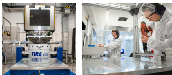
Fig. 1: Left: 89 kN Vibration Shaker with mounted Eu:CROPIS Structural Model; Right: Pyroshock test stand during a shock initiation
