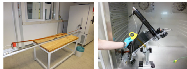
Fig. 18 Overview of the test setup for the "Engineering Tether pull-out test"
