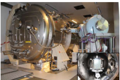
Fig. 6: Gossamer-1 EQM venting test setup, small vacuum chamber is vented into the already evacuated big space simulation chamber.
