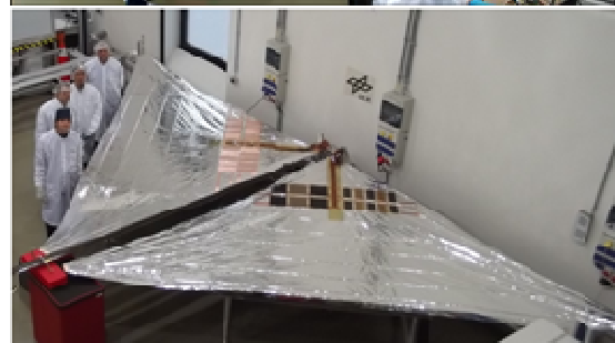
Fig. 8: Two sail segment deployed by the EQM of the deployment unit after the deployment test.
