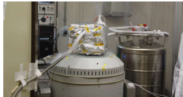
Fig. 22. Complete already cooled down test set-up with nitrogen tank
