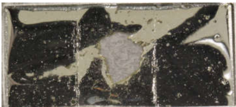
Fig. 13: Sample area exposed to space debris object (middle) as well as two artificially made folding lines, with negative (left) and positive (right) curvature.
