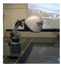
**Fig. 12** Robotic Motion Simulator at the DLR Institute of System Dynamics and Control [2].
