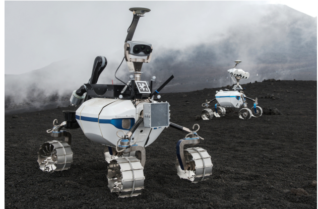
Fig. 1. The LRU rovers during the ROBEX Demo Mission Space at Mt. Etna. Front: LRU2 with manipulator. Back: LRU1 with Science Camera.
