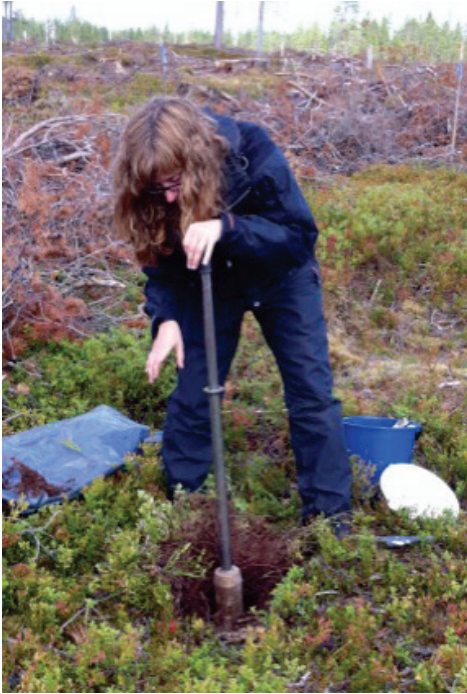
Figure 5. Sampling of the mineral soil with a sliding-weight core sampler at Rotflakamyran in 2012 (Photo: Annemieke Gärdenäs, SLU).
