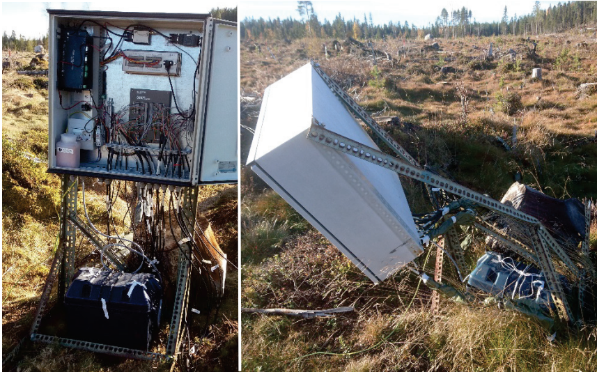
The logger station at Trågalidsberget before and after impact of a large mammal. Left photo: Linnea Hansson (2017-05-28). Right photo: Mikael Andersson (Skogforsk, 2018-10-10).
