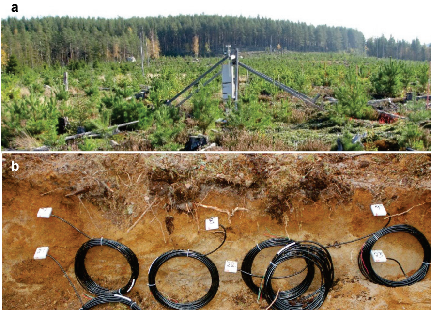
Figure 4. a) The centre of the Hagfors experimental site with the logger station, situated in the middle of the transect for soil temperature and water content measurements (photo: Linnea Hansson, September 2011). b) Soil profile and sensors installed at 20 and 45 cm from the original surface of the mineral soil before disc trenching. Microsites from the left: furrow, between furrows and furrow (photo: Eva Ring, Skogforsk, May 2006).
