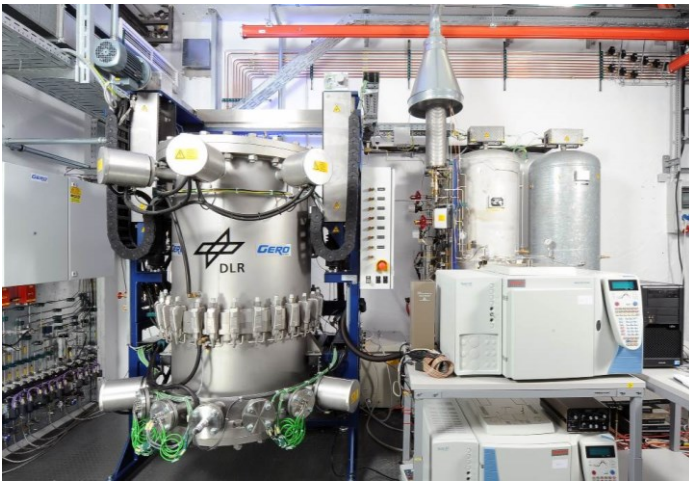
8 9 Figure 1: Pressurized SOC stack test facility of DLR.
