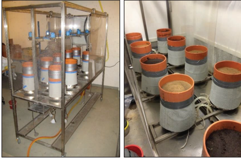
Figure 4. The rainfall simulator used in Paper I.
