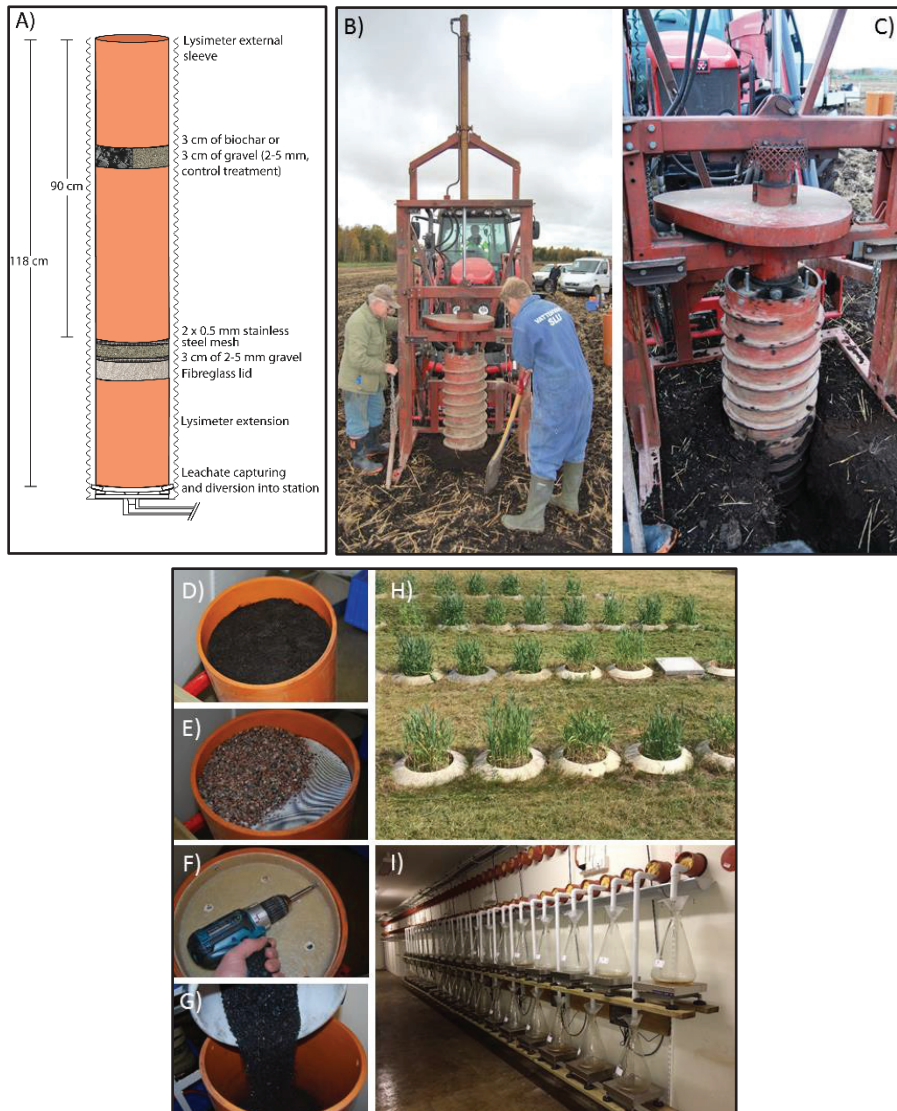
Figure 5. Lysimeter design with preparation steps. A) Lysimeter design; B and C), lysimeter excavation; D), bottom of lysimeter with gytja clay removed; E), addition of stainless steel mesh and 2-5 mm washed gravel; F), attaching the fiberglass lid; G), addition of biochar to the top of a lysimeter; H), lysimeters installed with wheat crop; I) leachate collection bottles in the lysimeter station.
