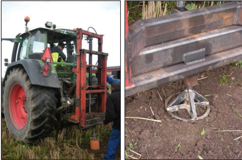
Figure 3. The rear mounted hydraulic soil column collection device in action. Photos: Mats Larsbo
