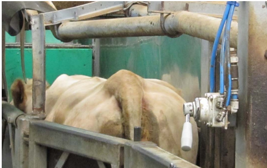
Figure 4. The stun box at the stationary slaughter plant, seen from behind. The guillotine gate at the entrance to the stun box is lifted. The animals fell from the shooting box to the right in the photo. (Photo: Anne Larsen, SLU)
