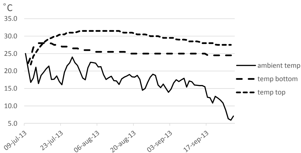
Figure 4 Ambient and in-silo temperature in the bottom (0,5 m) layer and top (1,90 m) layer.
