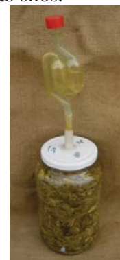
Picture 1. Glass jar silo with water-filled siphon on lid.
