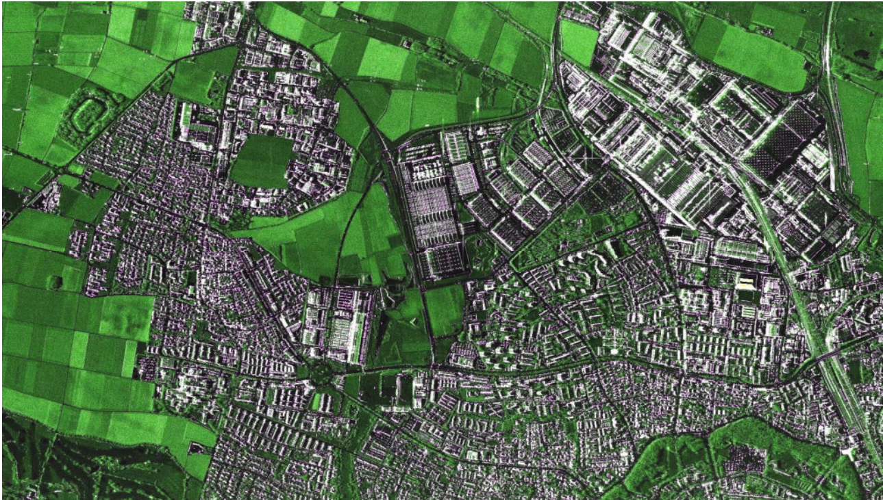
Figure 2.1-2 TerraSAR-X image of the north-western part of Ingolstadt and the Audi car factory acquired on January 11, 2018 in staring spotlight mode. The image covers an area of 5.4 km x 3.2 km at a range and azimuth resolution of 0.75 m and 0.21 m, respectively. The color coding is based on the local image statistics. After more than 11 years in orbit, TerraSAR-X continues to generate high-resolution SAR images of outstanding quality and without any degradation.
