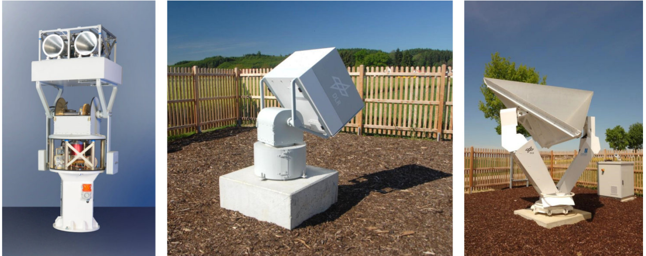
Figure 1.3-4 Calibration devices of the DLR calibration center: remote-controlled transponder in the laboratory (left) and deployed in the calibration field (center), and remote-controlled corner reflector (right) at one of the permanent sites within our calibration field covering a total area of 120 km x 40 km.
