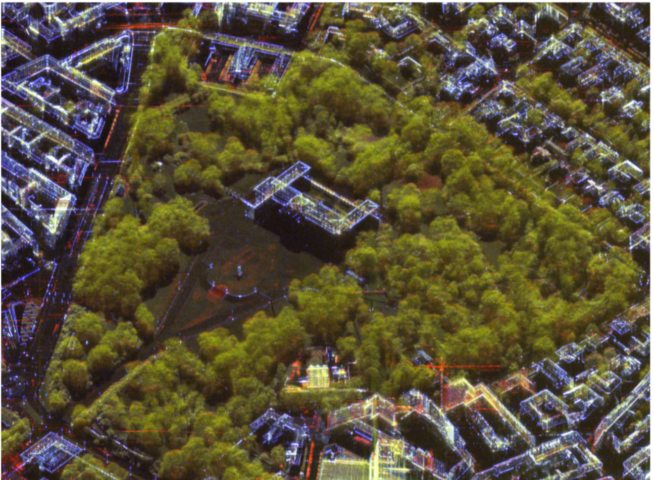
Figure 2.4-15 Exploitation of a series of 34 TerraSAR-X images of the Royal Palace in Oslo over 32 months: Color composite of SEPIA-filtered single images and pairwise coherence images. The bluish color indicates persistent scatterers, red shows strong amplitude change, and the greenish yellow color indicates coherency loss (mostly due to vegetation).
