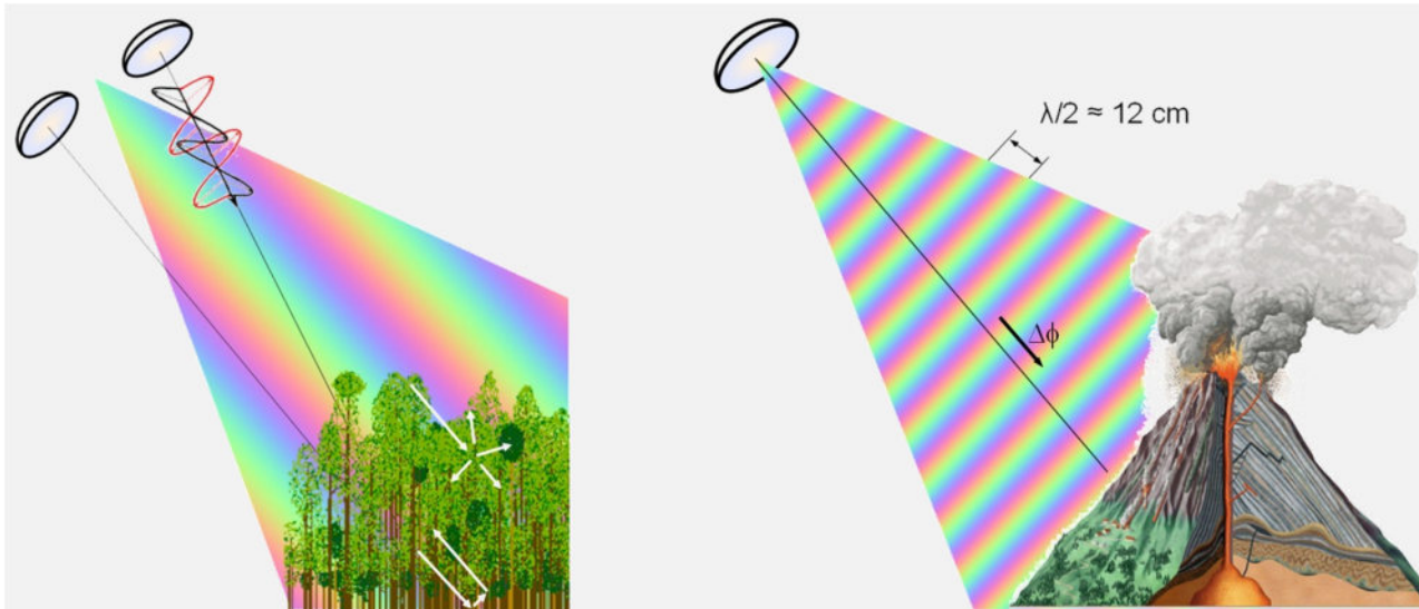
Figure 2.1-27 The two basic measurement modes of Tandem-L. Left: The 3-D structure mode employs polarimetric SAR interferometry and coherence tomography to measure tree heights and vertical vegetation profiles. The individual contributions from ground and canopy can be separated via their polarimetric signatures, and the corresponding heights can be measured by cross-track interferometry and multi-baseline tomography. Right: The deformation mode employs repeat-pass interferometry to measure surface deformations with millimetric accuracy.
