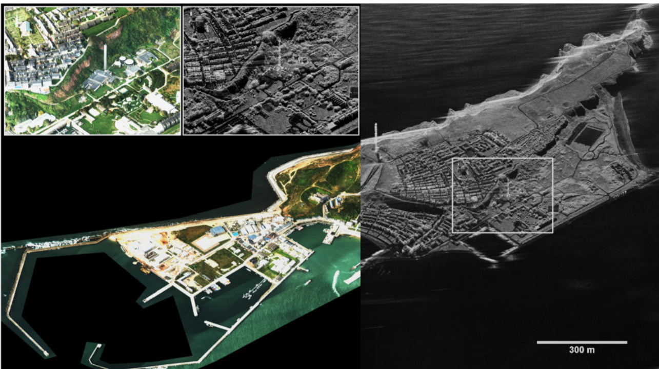
Figure 2.4-21 Sub-pixel accurate image fusion between an X-band F-SAR image and an optical image from DLR's airborne sensor system MACS for the whole island of Heligoland. The zoomed detail shows the outstanding accuracy even on a building level through the usage of a very accurate digital surface model.
