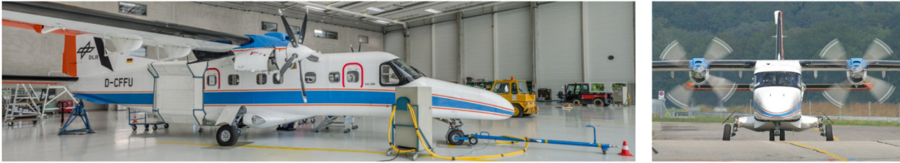
Figure 1.3-1 F-SAR sensor on-board the Dornier DO228-212 aircraft: at the hangar of DLR in Oberpfaffenhofen (left), starting for a flight measurement campaign (right).
