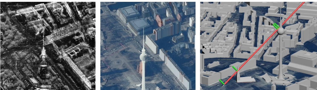
Figure 2.4-20 Image fusion between a TerraSAR-X image (left) and a Pleiades optical image (middle). The layover effect causing the TV tower to overlap with a church in the SAR image is visualized in a 3-D model (right).
