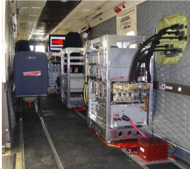
Figure 2.3-10 The DBFSAR racks mounted in the aircraft cabin during the maiden flight. The 6 waveguide connectors to the outside antenna configuration are visible on the right.
