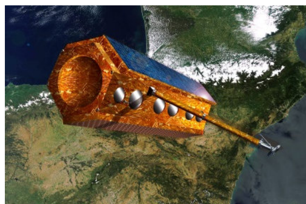
Figure 2.1-38 Artist's view of the PAZ satellite in orbit since February 22, 2018. Clearly visible are the microstrip patch radiators of the SAR antenna (lower surface), otherwise PAZ is a copy of TerraSAR-X.
