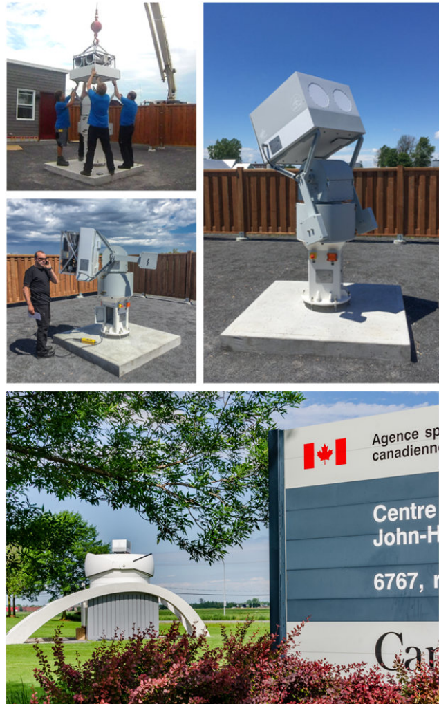
Figure 2.1-60 Installation of the C-band transponder system developed by the Institute for the Canadian Radarsat Constellation Mission featuring RCS of 64\text{ dBm}^2 at an absolute accuracy of 0.2 dB, RCS stability below 0.1 dB, and remote control (top). RCM transponder at CSA headquarters near Montreal, Canada (bottom).
