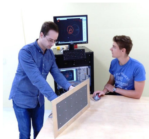
Figure 2.2-77 Top: elevation and azimuth patterns for H and V polarization in one diagram. The wider elevation patterns are pointing to 5 degrees off-nadir direction and show equally shaped patterns between -10 and 40 degrees. The narrower azimuth patterns are also in good accordance within the main beam area. Bottom: S-band antenna with 300 MHz bandwidth.
