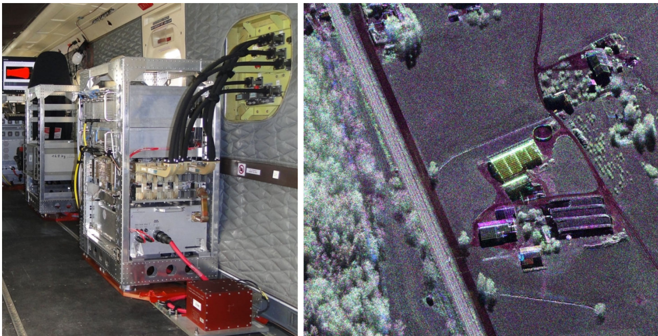
Figure 1.4-11 Left: DLR’s most recent airborne SAR sensor, the DBFSAR (Digital Beamforming SAR with up to 12 channels on receive), mounted in the cabin of the DO228-212 research aircraft. Right: polarimetric DBFSAR SAR image; X band, 20 cm x 20 cm resolution, magenta: VV, green: HV, blue: HH polarization.
