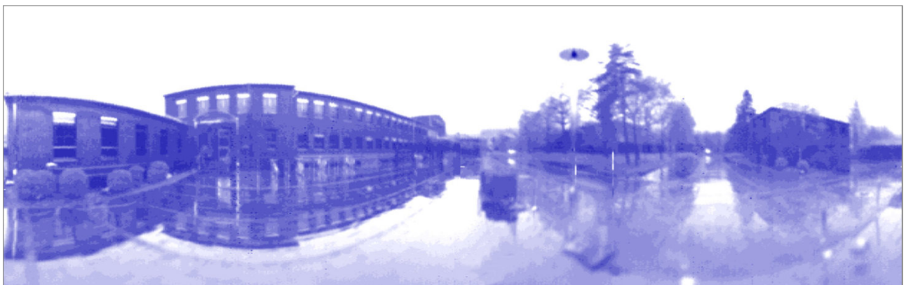
Figure 1.4-12 Panoramic image of the Institute for 360° azimuth angle scanning, acquired with the 90 GHz radiometer system ABOSCA. The image shows the Institute's main building on the left and the main entrance of the Oberpfaffenhofen site on the right. White color indicates cold brightness temperatures (down to 50 K) and dark blue color warm brightness temperatures (up to 300 K).
