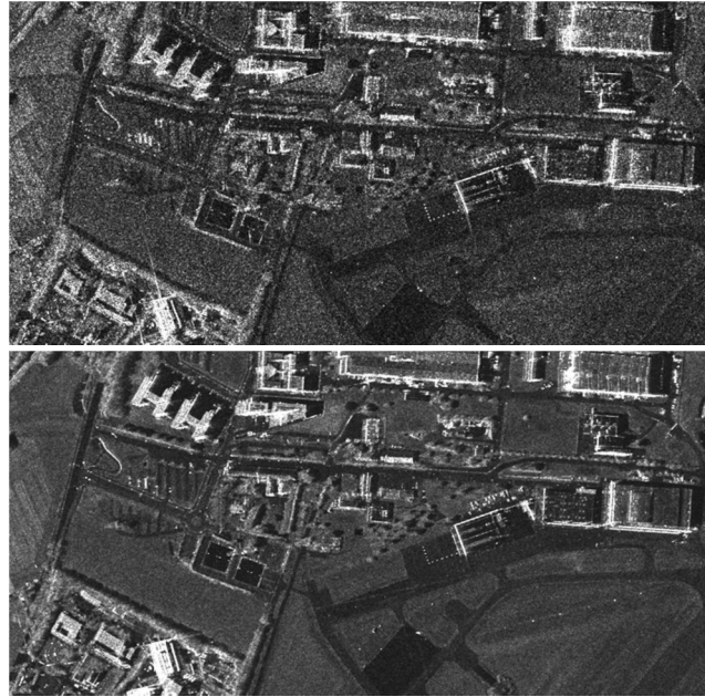
Figure 2.2-21 TerraSAR-X spotlight images acquired over Oberpfaffenhofen, Germany. The images are excerpts from larger images and show an area of 1000 m x 500 m. The upper image was acquired in nominal high-resolution sliding spotlight (HS) mode, while the lower image was captured in the new ultra-high-resolution staring spotlight (ST) mode. Both images were multilooked to the same resolution of 1 m x 1 m. The improvement in speckle reduction due to the larger multilook factor is evident for the new ST mode.
