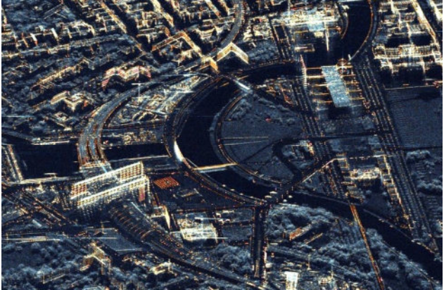
Figure 2.1-3 Staring spotlight acquisition over the political center of Berlin, Germany. Very fine details such as the corners of the main station’s steel construction or lightning rods become clearly visible at a resolution of 1 m in ground range and 0.21 m in azimuth. The image is multilooked to 1 m x 1 m and artificially color-coded.
