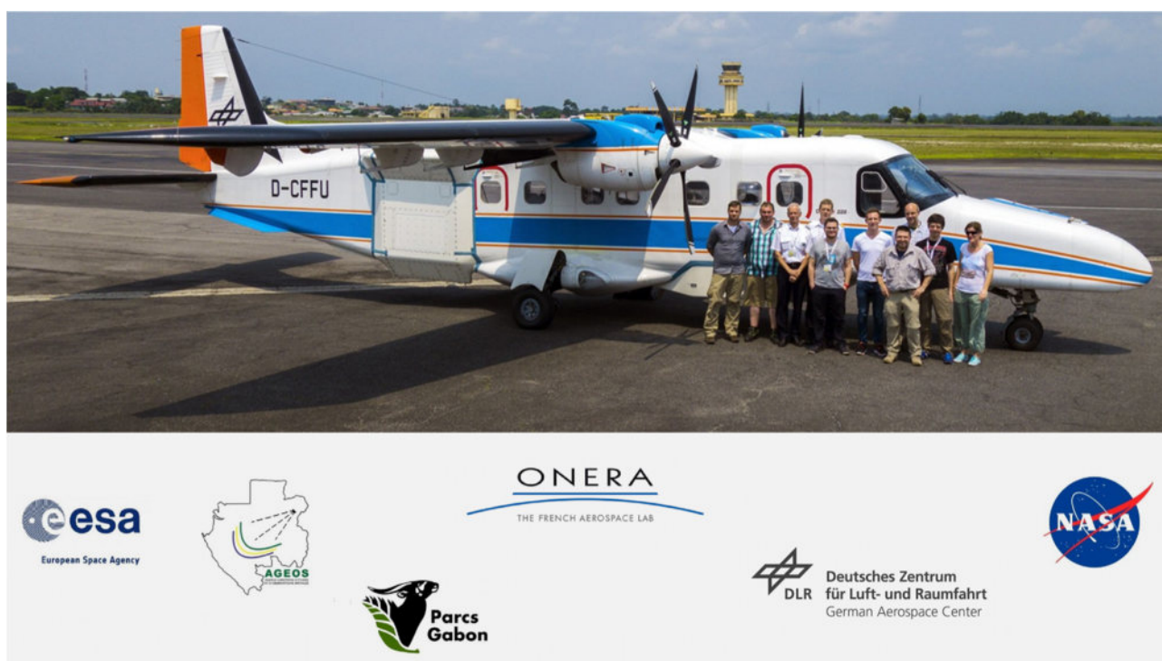
Figure 2.3-20 The AfriSAR team together with ESA's project coordinator in front of DLR's DO228-212 research aircraft at Libreville airport in Gabon. The radar antenna carrier is clearly visible on the side of the aircraft behind the wing.
