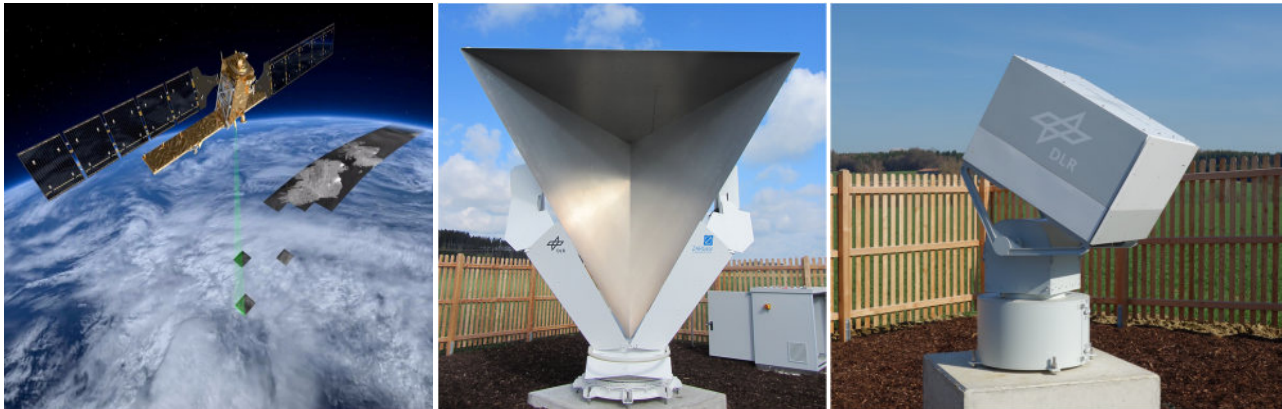
Figure 2.1-43 Sentinel-1, ESA’s C-band satellite as part of the Copernicus Program (left); DLR’s remote controlled corner reflector (center) and transponder (right) deployed and operated for Sentinel-1
