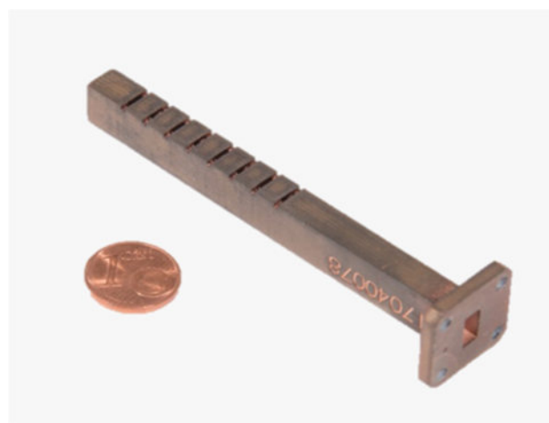
Figure 2.2-81 Ka-band slotted waveguide antenna prototype out of 3-D printed plastic metalized with copper
