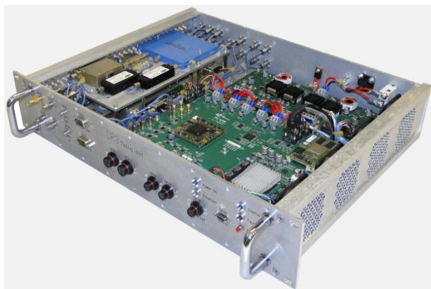
Figure 2.3-6 The high-precision DBFSAR timing unit featuring a GPS synchronized rubidium atomic clock with a frequency stability better than 5 \cdot 10^{-12} per year.
