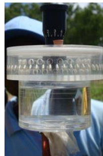
Figure 15. Andersson evaporimeter. (Photo: Mário Chilundo)
