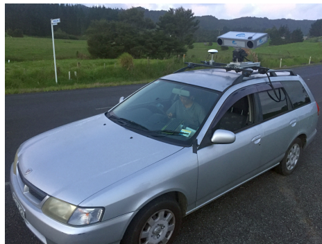
Figure 1: Used test vehicle on Otaika Valley Road. IPS setup during the measurement campaign. A GNSS antenna of a reference receiver is located left of the IPS-sensorhead.
