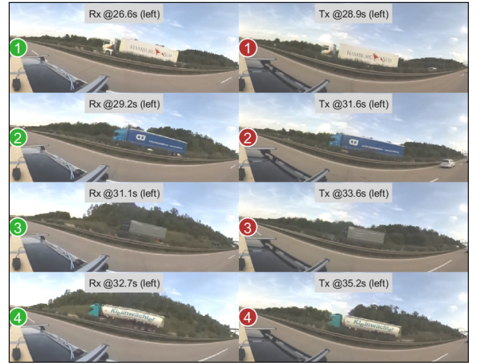
Fig. 4 TX and RX drive at a constant distance, one behind the other, 4 trucks in oncoming direction (see Fig. 3)
