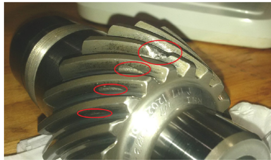
Fig. 14. Left input pinion with a chipped tooth and pitted surface areas circled in red. (For interpretation of the references to colour in this figure legend, the reader is referred to the web version of this article.)
