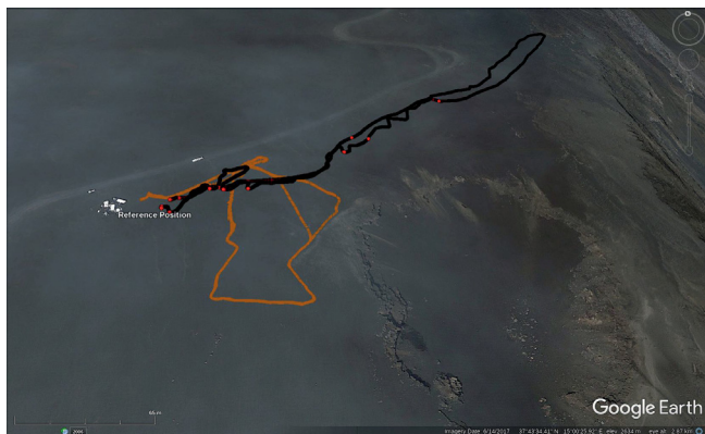
Figure 4 Trajectories of the long range navigation tests plotted with Google Earth using the DGPS ground truth data; length of the trajectory of dataset 1 (brown) is approximately 834 m and of trajectory of dataset 2 (black) is approximately 1097 m
