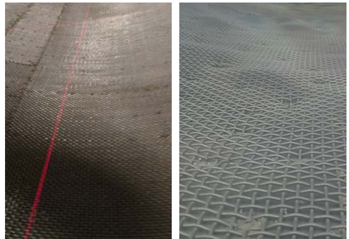
FIGURE 9: WIRE-MESH RECENTLY INSTALLED (LEFT) AND AFTER APPROX. 30 H OF ON-SUN OPERATION (RIGHT)
