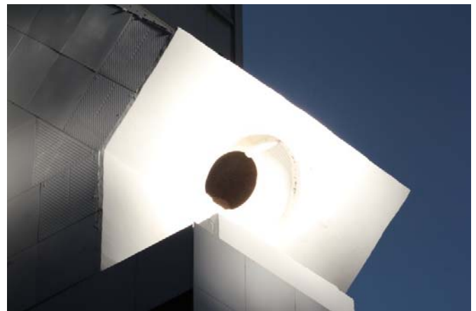
FIGURE 6: VIEW OF RECEIVER DURING ON-SUN OPERATION
