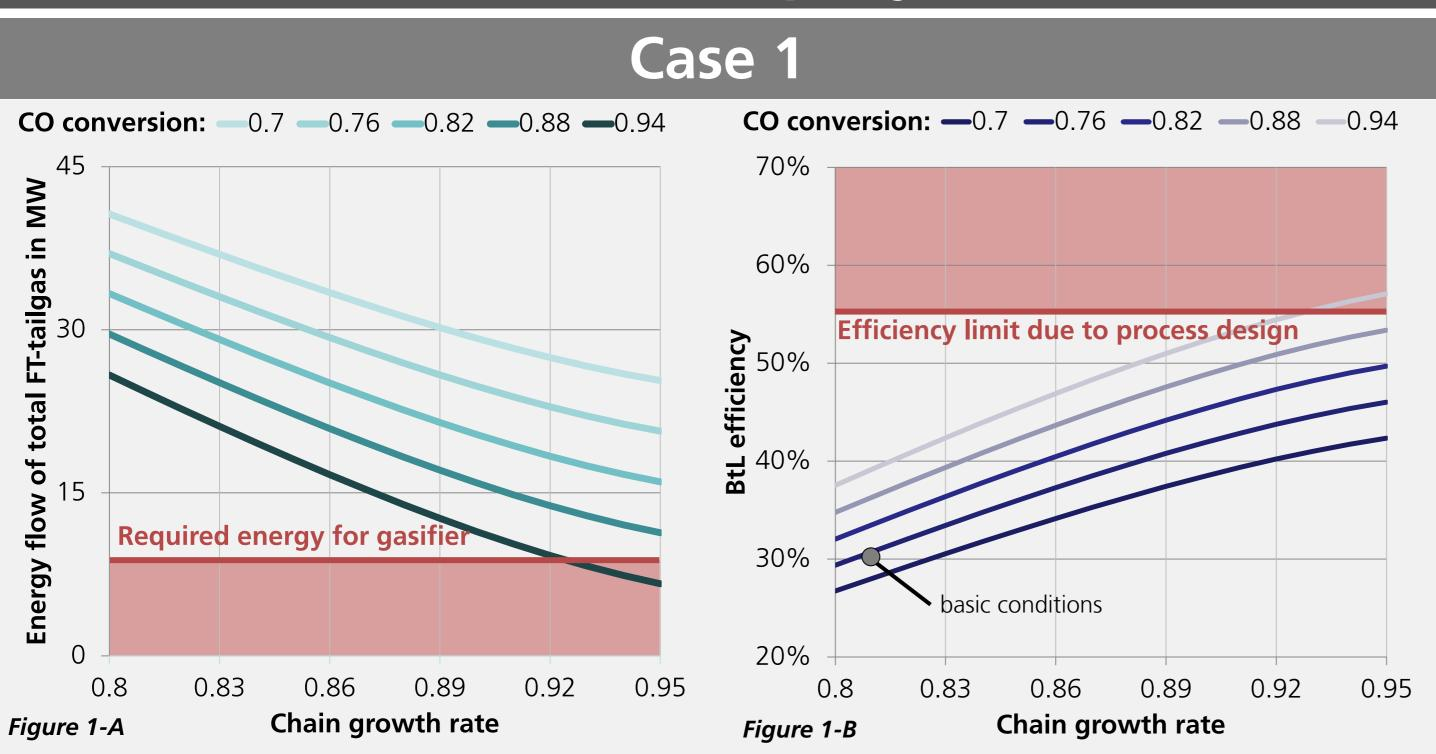
The **red** line in Figure 1-A indicates how much energy the FT-tailgas needs to contain to provide the required amount of heat in the DFB
