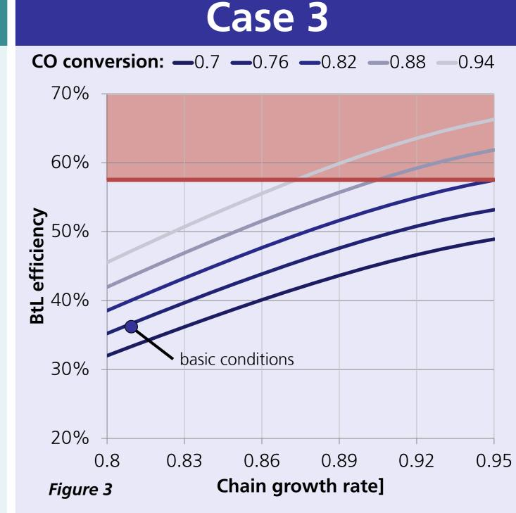
Allothermal reforming allows the FT synthesis to work less effective and still achieve the same maximum BtLefficiency as case 2
