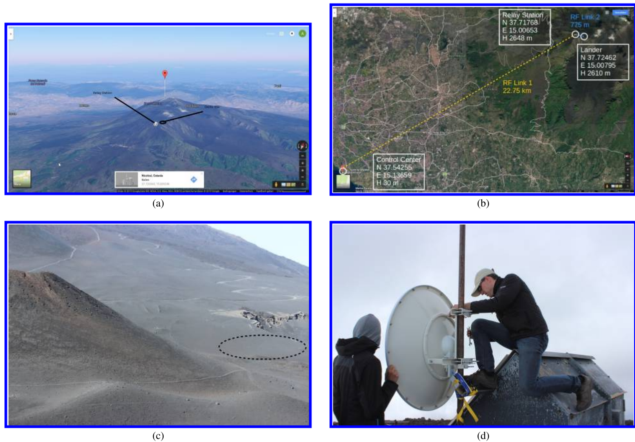
Fig. 2 (a) Perspective view on mount Etna. (b) Map of the entire area with the RF relay and coordinates of control center, relay station and lander. (c) View from La Montagnola towards test site marked by an ellipse. (d) Installation of a relay antenna (RF Link 1) on La Montagnola.
