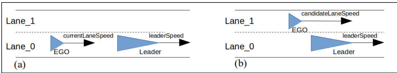
Figure 6. (a) The ego vehicle is in the car-following mode behind a bus. (b) The ego vehicle performs a tactical lane-change to gain speed.
