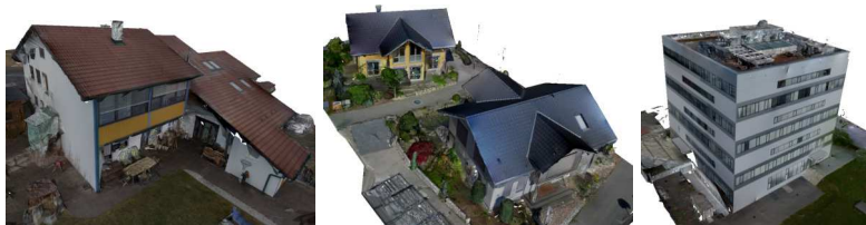
Fig. 1. Results of the proposed approach textured with [33]. One can observe that planar parts in the scene (facades, windows, roof) are represented by planar surfaces and building edges where two facades intersect each other are represented by straight lines. Note that holes in the model are due to missing visibility information during texturing.
