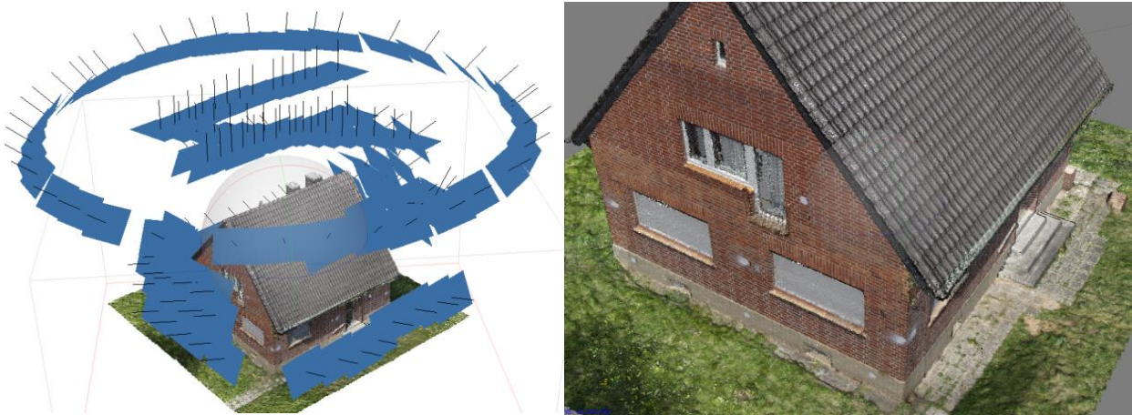
Figure 5: Camera positions for the selected subset of nadir, oblique and near-horizontal images as calculated by Agisoft Photoscan (left), 3D point cloud with very high detail (approx. 12 million points, right)
