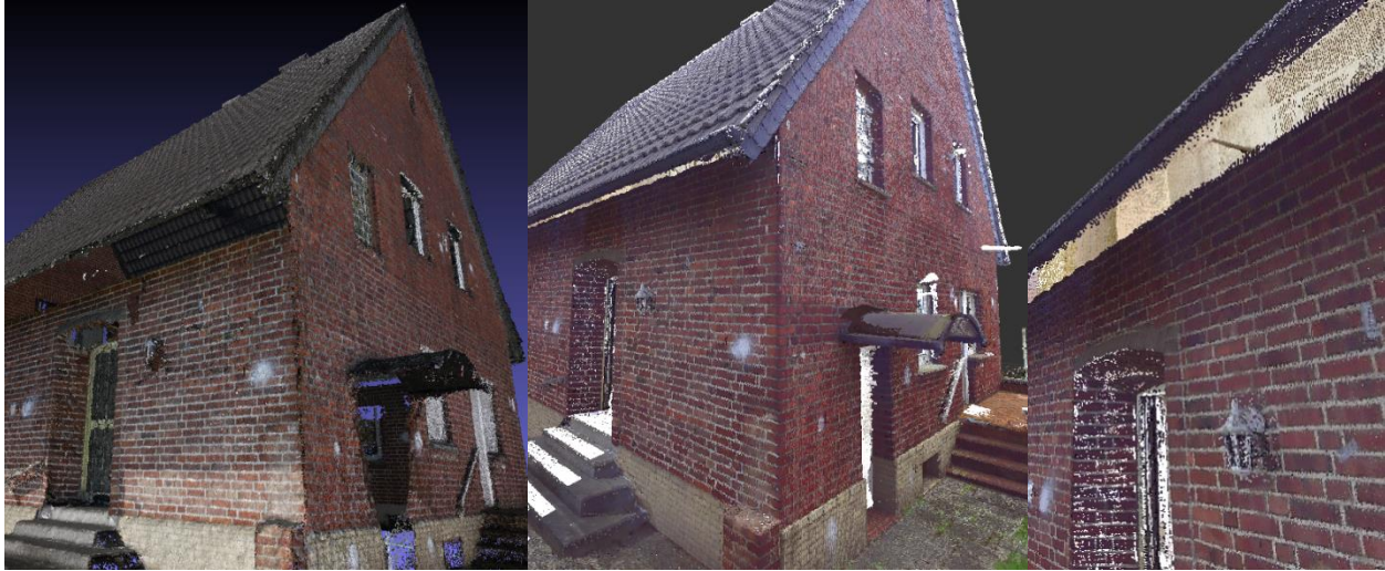
Figure 6: Blind spaces below roof overhangs and canopies in photogrammetry-based point cloud (left) and the respective regions in laser scanner point cloud (middle, right)
