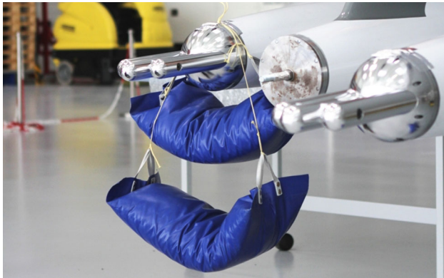
Fig. 25 Strain gauge calibration of a PMS carrier
