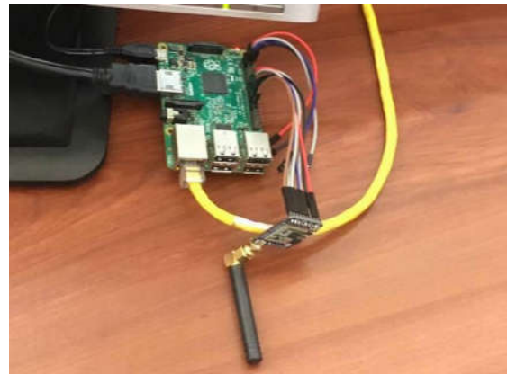
Fig. 14. Raspberry Pi 3 and RFM69HCW module used to collect scientific data.
