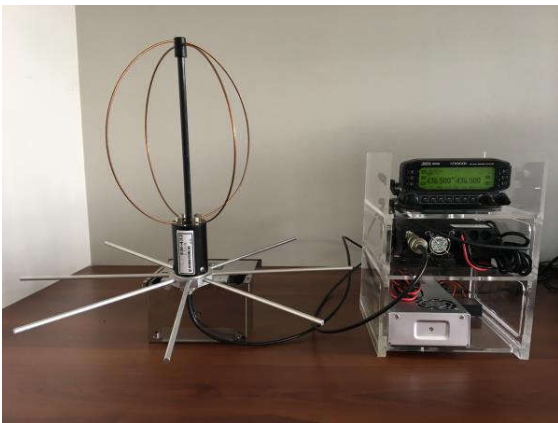
Fig. 13. M2 Inc. EB-432 antenna and Kenwood TM-D710G used to run the ground station for Project Irazú.
